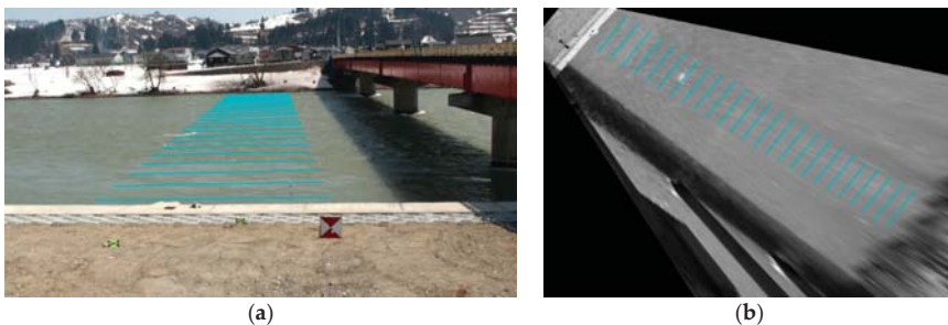
Figure 1. Example of an ortho-rectified image (b) for an image (a) obtained by using a normal high definition video camera, each with search lines.
