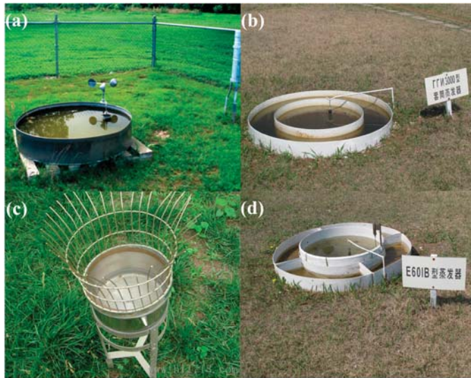
Figure 1. Four types of evaporation evaporimeters: Class A from the USA (a); GGI-3000 from Russia (b); and ϕ20 (c) and E601B (d) from China.
