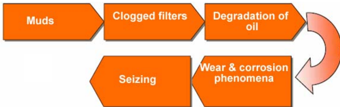
Figure 22: Contamination by water
