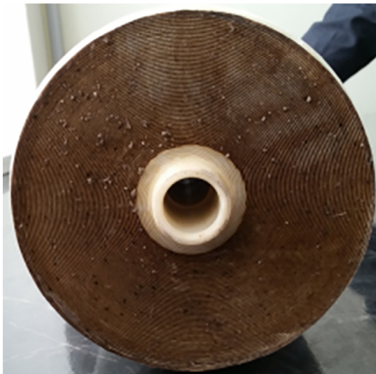
Figure 3.4 Bio-fouled spiral-wound RO membrane.
