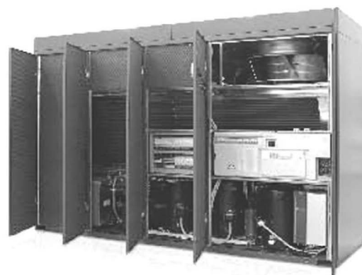
Figure 7.57. Precision air conditioning unit supplies air to the raised floor plenum from where it is supplied to the cold aisle. Cooled air flows via data racks to the hot aisle from where it is sucked to the air intake of precision air conditioning unit.
