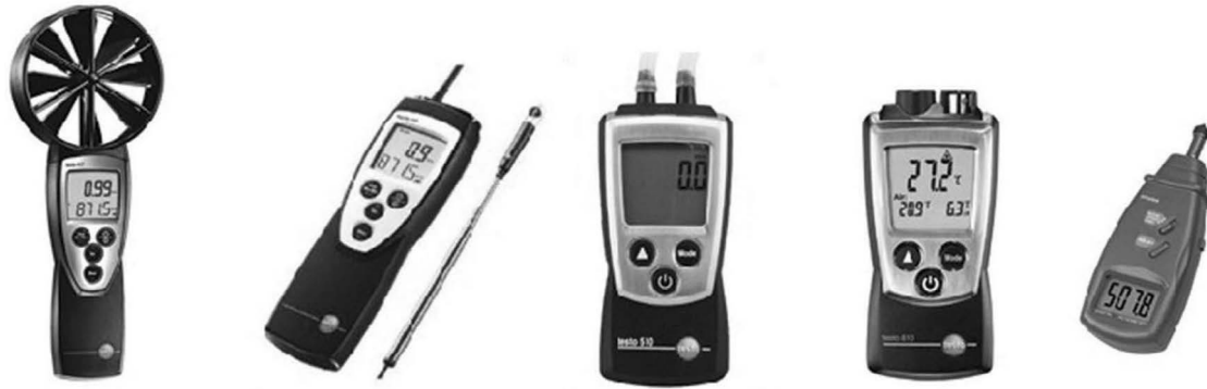
Figure 7.13. Vane anemometer, hot wire anemometer, differential pressure meter, air and surface temperature meter as well as tachometer are required to measure the performance of an air handling unit.
