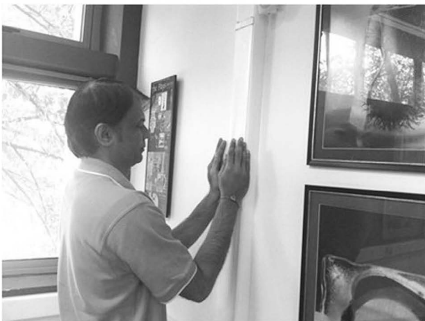
Figure 3.16. During the Functional Performance Testing, there is a need to artificially alter the conditions around measurement sensors.
