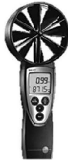
Figure 7.13. Vane anemometer, hot wire anemometer, differential pressure meter, air and surface temperature meter as well as tachometer are required to measure the performance of an air handling unit.
