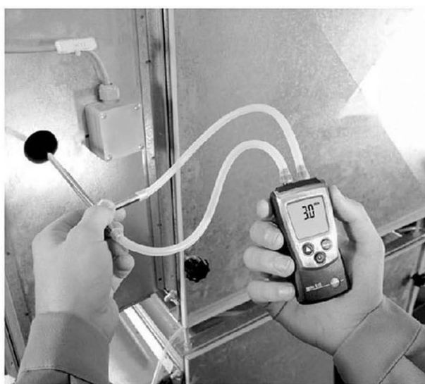
Figure 7.6. As air flow is turbulent inside the duct, there is variation in the velocity over the face area of a duct. This is why the average of several velocity measurement readings gives more accurate result. Air flow measurement can be done either using hot wire anemometer (velocity measurement) or pitot tube (pressure measurement). Typical duct velocities are 1-15 m/s (instrument resolution is typically 0.1 m/s). Pitot tube readings with the same velocities are 2-50 Pa (instrument resolution is typically 1 Pa). Therefore, the accuracy of the pitot tube measurement is poorer with low velocities.
