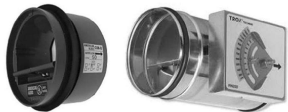
Figure 7.24. There are two basic models of system powered constant volume dampers: one to be installed inside the duct (left) that has typically only one preselected air flow rate and the other one (right) in which the air flow rate can be re-adjusted.
