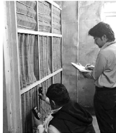
Figure 7.14. AHU air flow rates are typically measured in front of the filter section using the vane anemometer. As the air flow rate is not even in the filter section, several points shall be measured.
