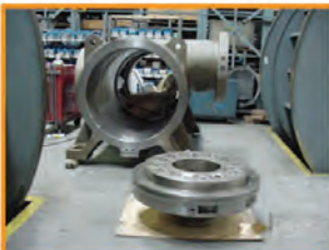
Figure 5-1. Assembly of a compressor utilizing modular design.
