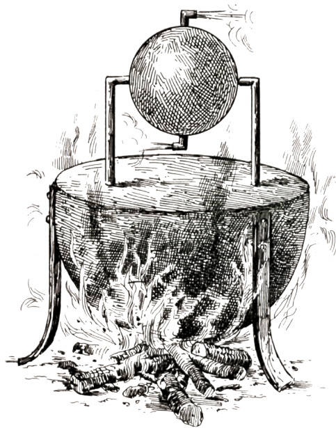
Figure 0-2. Aeolipile, Heron of Alexandria 150 B.C.E.
