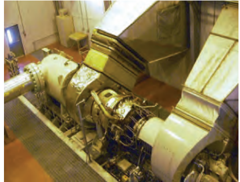
Figure 7-4. Compressor driven by a two-shaft gas turbine
