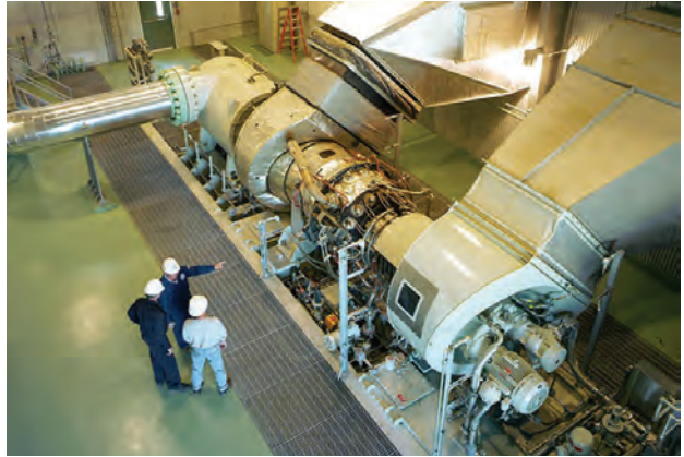
Figure 0-5. Titan 130 2-shaft gas turbine driving a Solar compressor.
