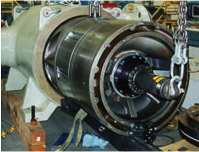
Barrel Type Casing - Horizontally or vertically split bundle
