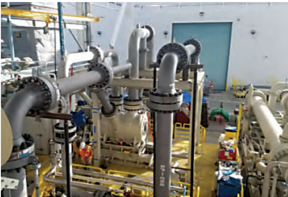
Figure 10-1. Titan 130 driven C41D closed-loop validation testing, San Diego.
