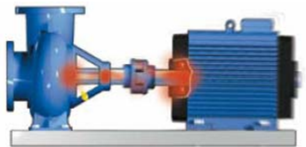
Figure 58: Heat generated by an alignment defect
