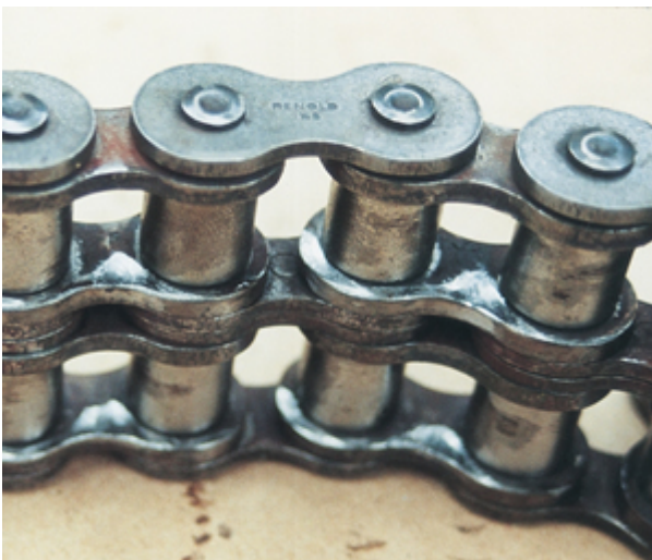
Figure 168: Poor lubrication and misalignment
