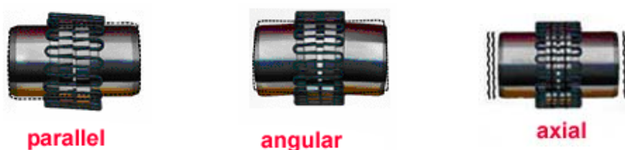
Figure 33: Detail of the possible misalignments
