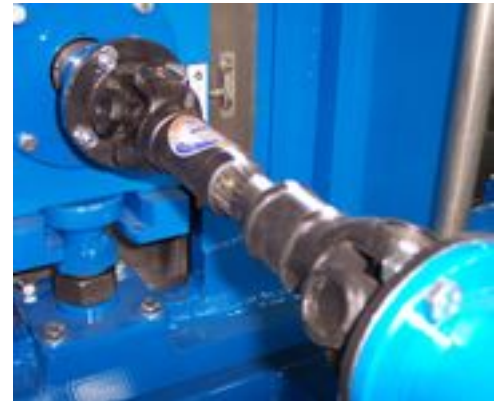
Figure 49: Universal joints in an installation
