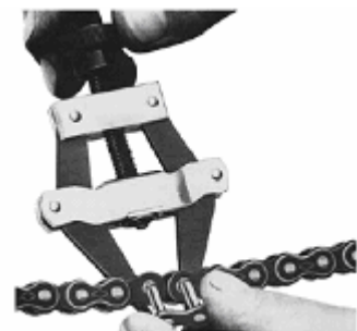
Figure 125: Quick release link (a spring in this case) and chain link pliers
