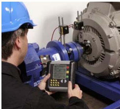
Figure 60: Laser alignment method
