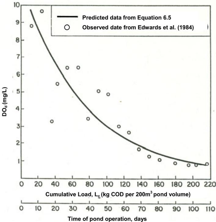
Figure 6.13 Cumulative load versus  $\text{DO}_d$  for 100 kg COD/(ha-day) loaded septage ponds
