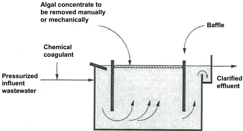
Figure 5.12 Schematic of a dissolved air flotation unit
