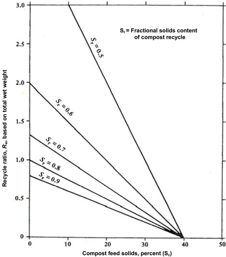
Figure 3.5 Effect of compost feed solids content on the wet weight recycle ratio needed to achieve a 40% mixture solids content (Haug 1979; reproduced by permission of the Water Pollution Control Federation USA)
