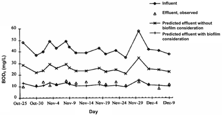
Figure 7.13 Predicted and observed effluent BOD<sub>5</sub> concentration of the WHP (Polprasert and Khatiwada 1998)
