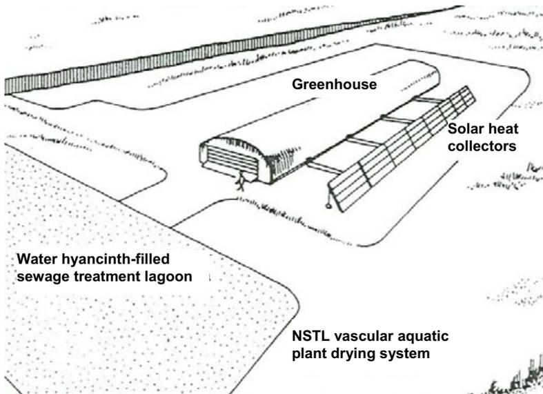
Figure 7.7 Solar energy being harnessed to dry aquatic weeds at the National Space Technology Laboratories (NSTL) near Bay St. Louis, Mississippi (NAS 1976). Note: this system is connected to a lagoon full of water hyacinth growing in sewage effluent.
