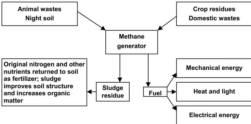
Figure 4.1 Impact of anaerobic fermentation on use of organic wastes (NAS 1977)
