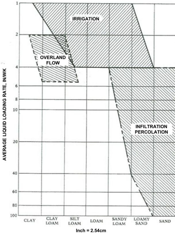
Figure 8.1 Soil type vs liquid loading rates for different load application approaches (U.S. EPA 1976)
