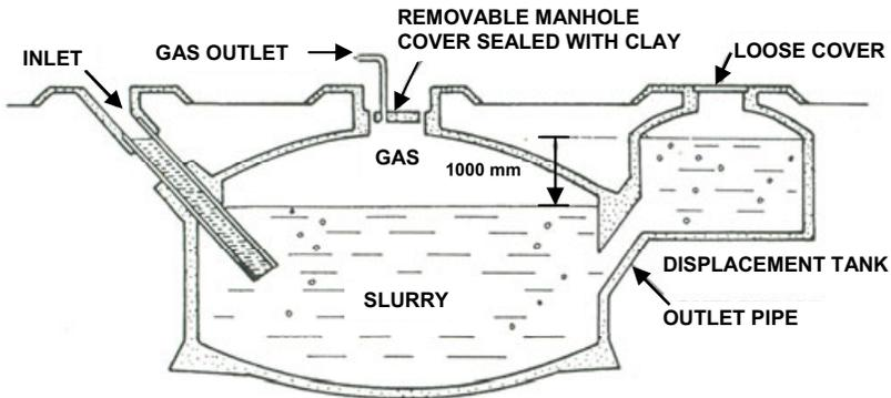
Figure 4.5 Fixed-dome digester
