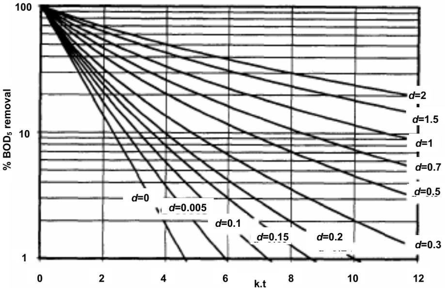
Figure 7.14 Design chart for BOD<sub>5</sub> removal in water hyacinth ponds (Polprasert *et al.* 1998)
