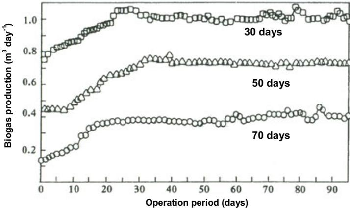
Figure 4.8 Mean daily biogas production at hydraulic retention times of 30, 50, and 70 days from pilot small-scale digesters. Each point is the mean of four digesters.
