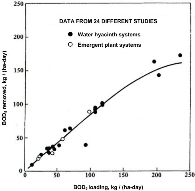
Figure 7.15 BOD removals as a function of BOD loading in aquatic systems (after Stowell *et al.* 1981; reproduced by permission of the American Society of Civil engineers)
