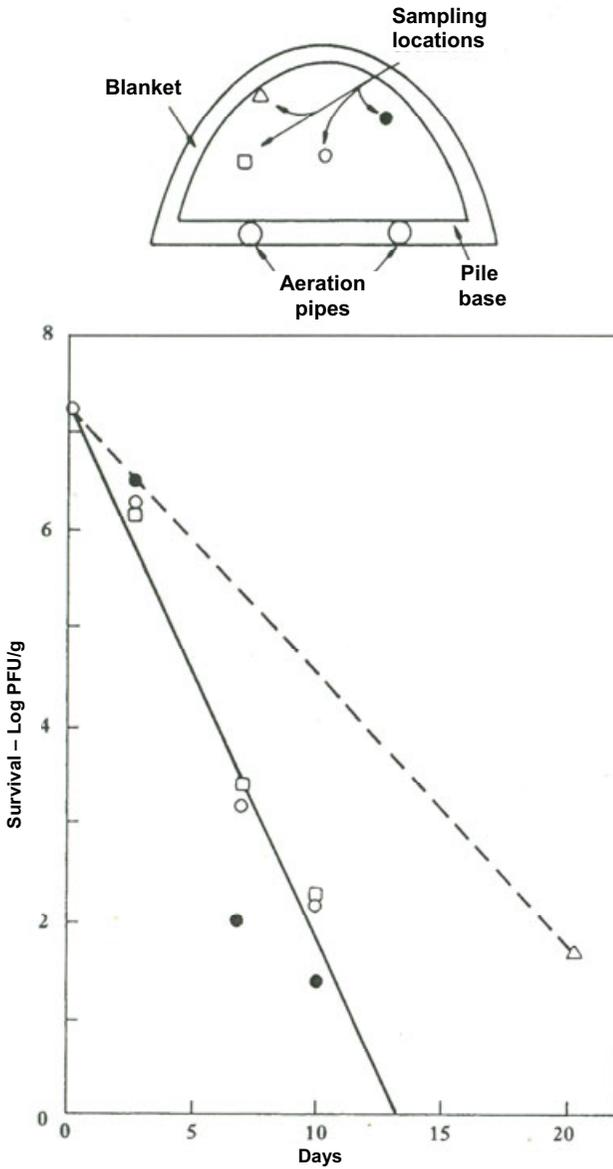
Figure 3.21 Destruction of  $F_2$  bacteria virus during composting by the BARC system (U.S. EPA 1985)
