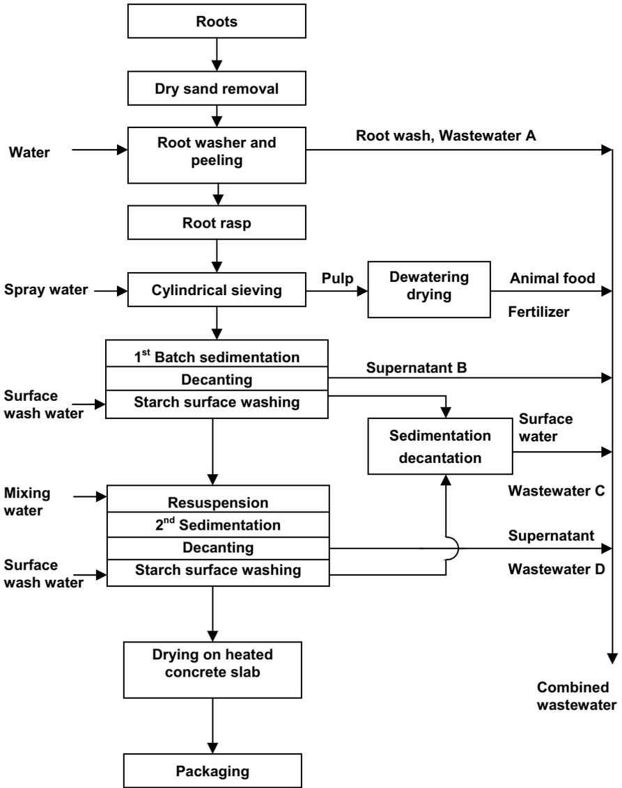
Figure 2.3 Second-grade tapioca processing (Thanh 1984)
