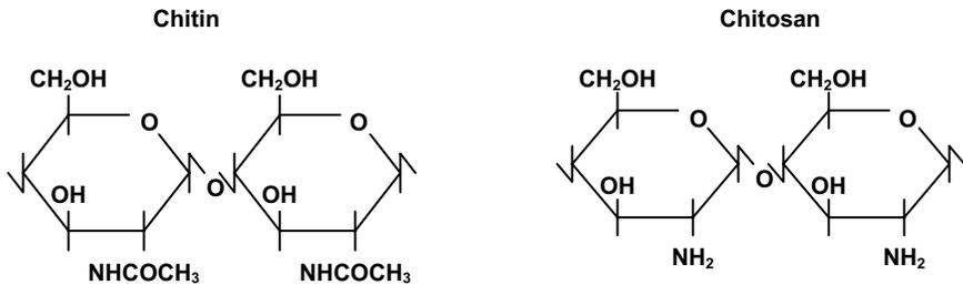
Figure 6.16 Chemical structures of chitin and chitosan
