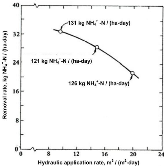
Figure 7.16  $NH_4^+-N$  removal as a function of hydraulic application rate (corresponding loading rates for  $NH_4^+-N$  are as shown) (after Weber and Tchobanoglous 1985; reproduced by permission of the Water Pollution Control Federation, USA)
