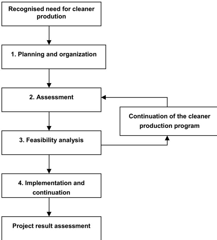
Figure 2.11 Four principle steps of cleaner production
