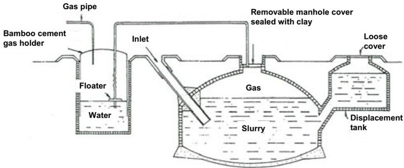
Figure 4.12 Fixed-dome digester with separate gas holder
