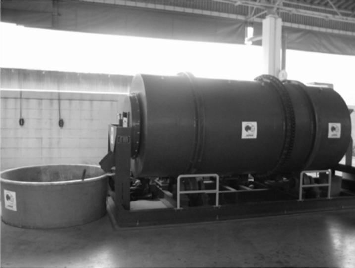
Figure 3.19 Aerobic composting unit for a small community, Thailand
