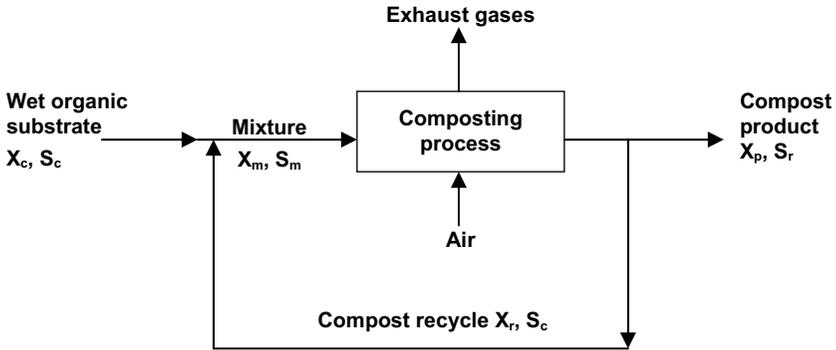
Figure 3.4 Schematic mass balance diagram for sludge composting showing inputs of compost feed and compost recycle, and compost product (adapted from Haung 1979; reproduced by permission of the Water Pollution Control Federation USA)
