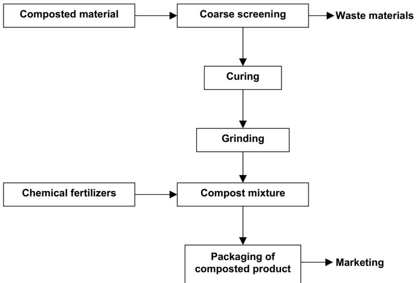
Figure 3.22 Flow chart of compost fertilizer production process
