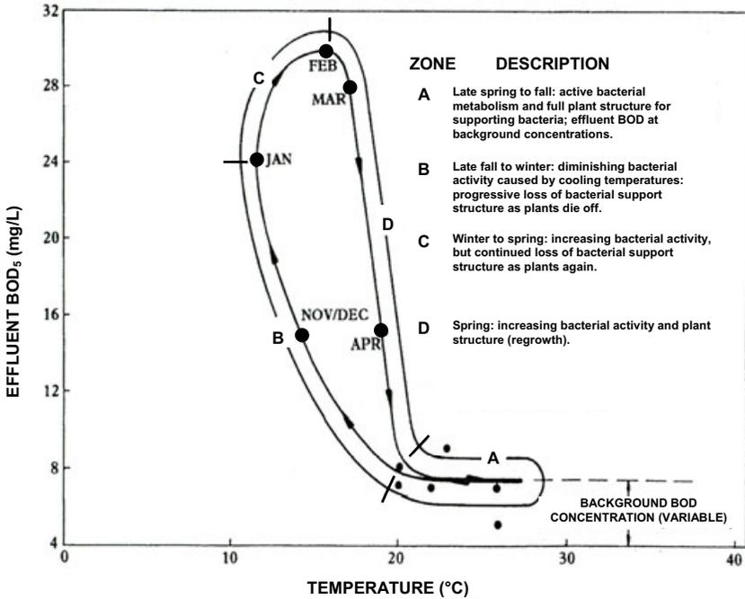
Figure 7.11 An example of the seasonality of effluent BOD<sub>5</sub> concentrations. *Note:* Compiled by Stowell *et al.* (1980), using data from Wolverton and McDonald (1976a). Reproduced by permission
