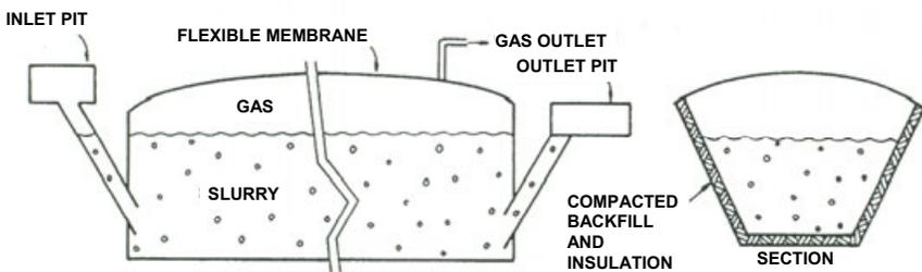
Figure 4.10 Plug-flow digester
