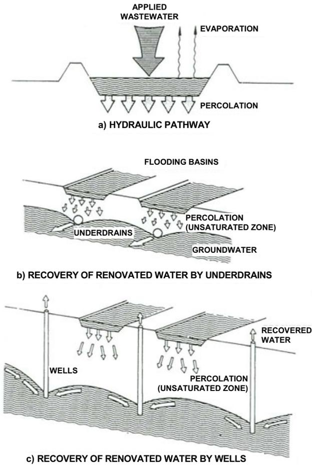
Figure 8.3 Rapid infiltrations (U.S.EPA 1981)
