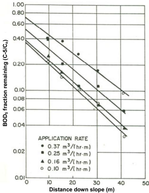
Figure 8.9 BOD<sub>5</sub> fraction remaining versus distance down-slope; application rate study with screened raw wastewater (Smith and Schroeder 1985)
