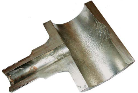
Evidence of erosion by droplets from the nozzle into the tube (internal surface).
