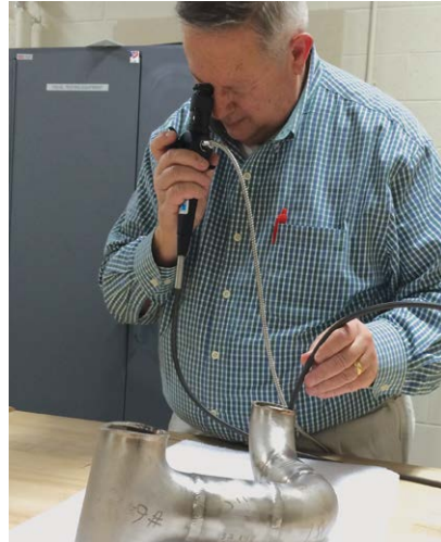
Fiber optic borescope in use.
