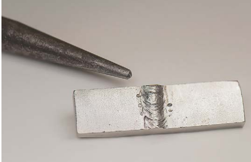
Tool marks from the pointed end of a weld chipping hammer. (Allgaier)
