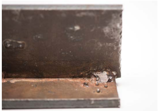
Weld spatter. (Allgaier)
