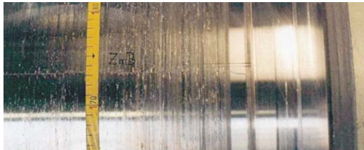
Part of a rotating machine showing wear (phonographic groove in appearance).
