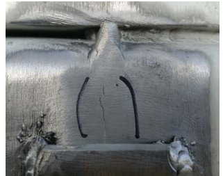
Close-up of a crack in ground flush weld behind cover plate. (Siderius)
