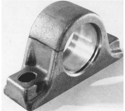
Indication of cold shut in a casting, enhanced here with magnetic particles.
