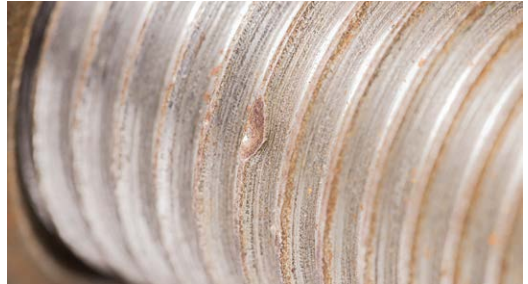
Mishandling tool strike from a hammer in bolt threads (round edge or ball end of hammer strike could prevent nut travel). (Allgaier)
