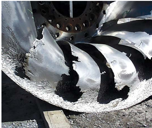
Cavitation wear in turbine blades.
