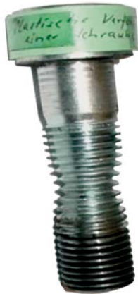
Bolt showing deformation (necking down).
