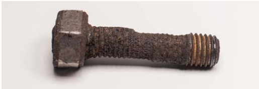
General corrosion of a bolt. (Allgaier)
