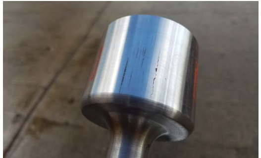
Inclusions in bar stock exposed during machining are visible following machining. (Siderius)
