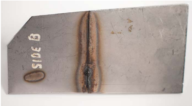
Excessive oxidation. (Allgaier)
