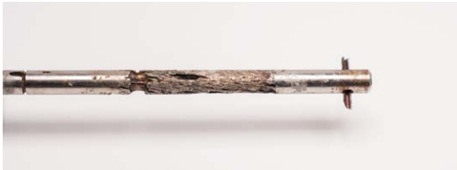
Intergranular corrosion cracking of a chlorinated water valve stem (swimming pool). (Allgaier)
