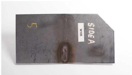
Heat-treating discoloration. (Allgaier)
