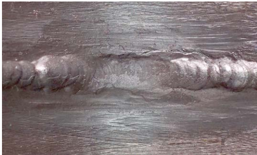
Concave weld at inside diameter of pipe-to-pipe weld.
