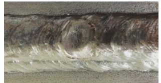
Visual appearance of a crater crack.
