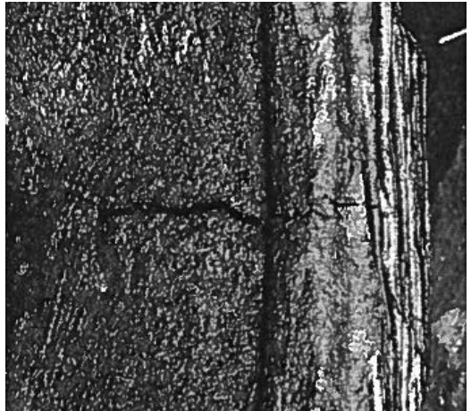
Visual appearance of hot tears in a casting.
