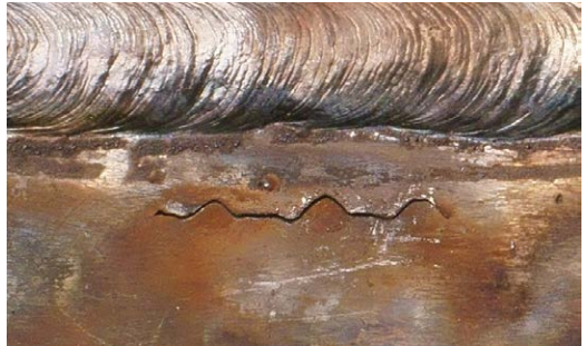
Visual appearance of heat-affected zone crack.
