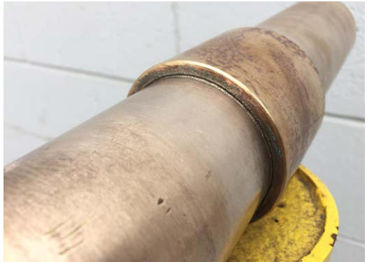
Braze sample showing inadequate fillet. (Inspection Testing)
