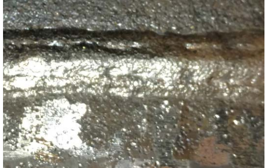
Excess needle gun marks. (Vona)
