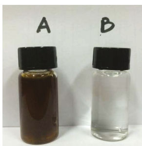
Figure 7. Images of original organic fertilizer sample (A) and MD permeate sample (B).
