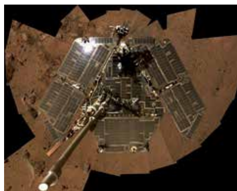
Fig. 4. Using of multijunction solar cells for Mars rover missions 1 .
