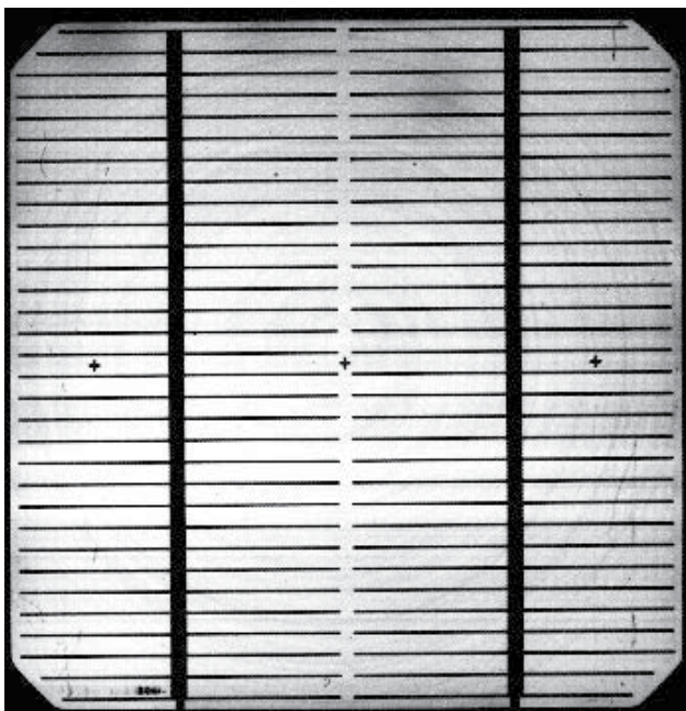
Fig. 11. Analyses of output local current of the sample no. 3 by usage of focused LED diode with middle wavelength 430 nm (blue LED, T=297 K)
