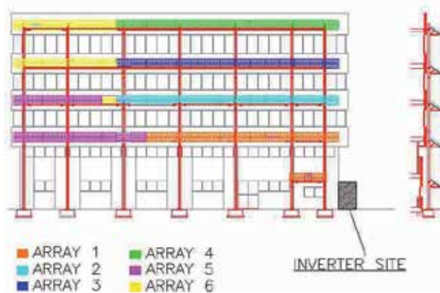
Fig. 22. PV arrays on the façade of the 1 st system.
