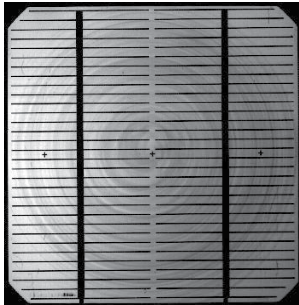
Fig. 9. Analyses of output local current of the sample no. 1 by usage of focused LED diode with middle wavelength 560 nm (green LED, T=297 K)
