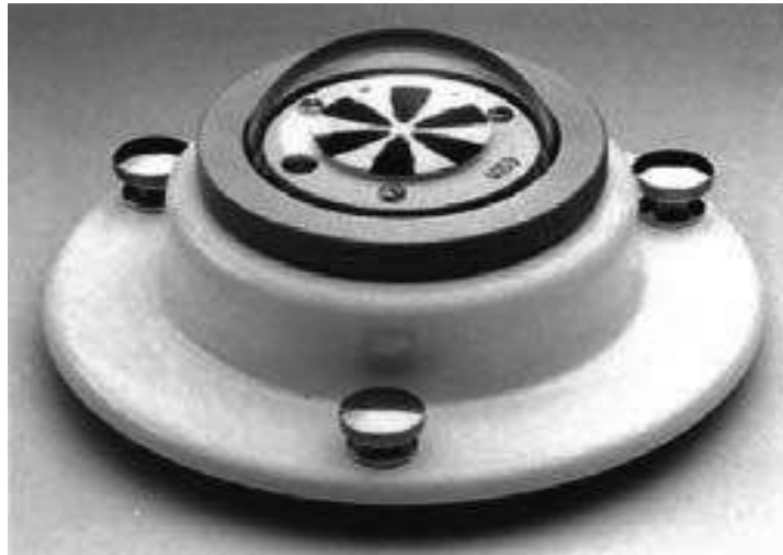
Figure-14: (a) A thermopile-type, black-and-white pyranometer (also known as 'Eppley' Pyranometer in USA )
