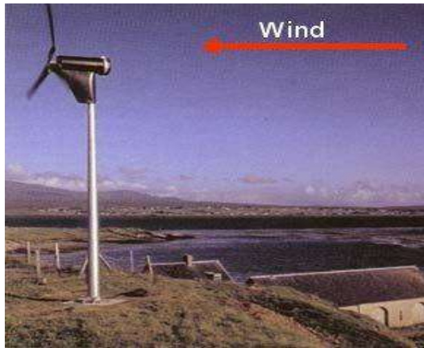
Figure-8: Downwind wind Turbine
