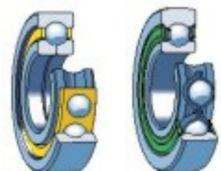
Figure 50: Bearings with one row of balls
