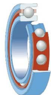
Figure 53: Angular contact bearing with one row of balls
