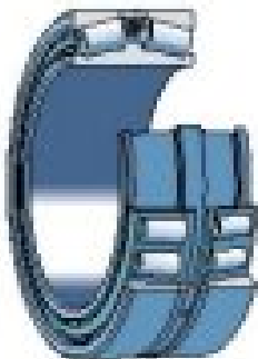
Figure 65: Two-row tapered roller bearing
