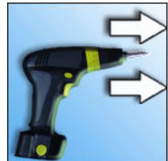
Figure 9: Example of an axial load: power drill
