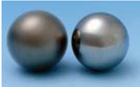
Figure 162 : Ball after passing of an electric current
