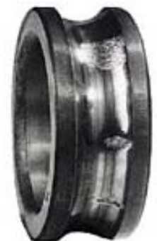
Figure 161: Chipping of an inner bushing further to incorrect installation
