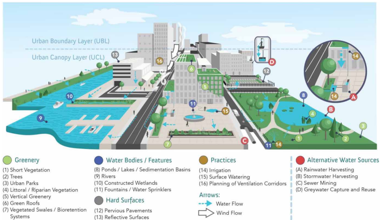
Figure 3 | Blue Green Systems and other measures (reflective surfaces) for urban heat mitigation. Blue Green Systems include Blue Green Infrastructure (greenery and water bodies/features), some hard surfaces and practices that ensure space and water availability for enhanced cooling.
