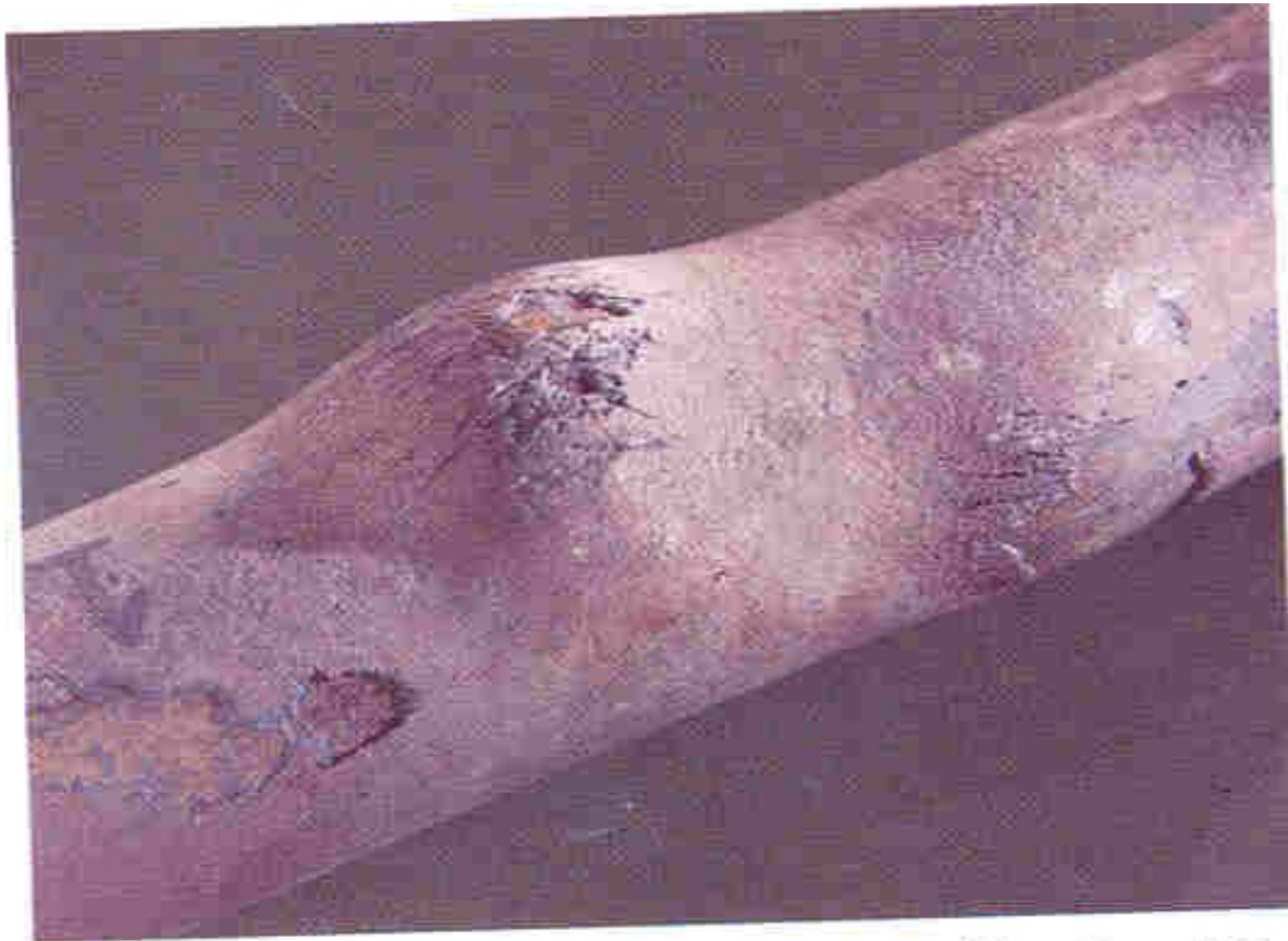
Figure 14-2. Deposit accumulation restricted heat transfer, leading to long-term overheating.
