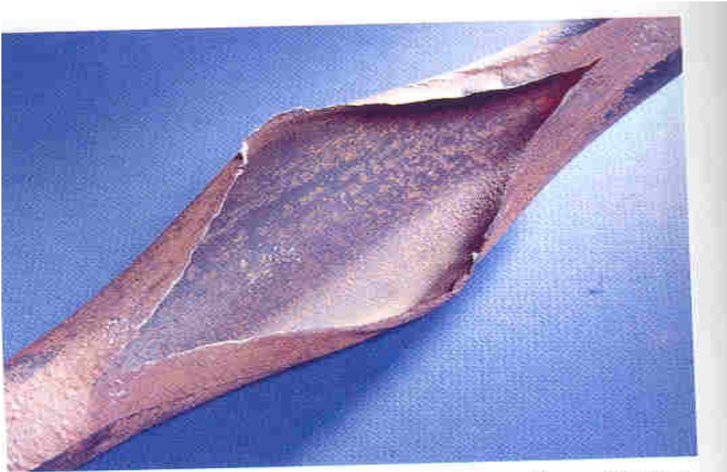
Figure 14-3. Thin-lipped burst caused by rapid overheating.
