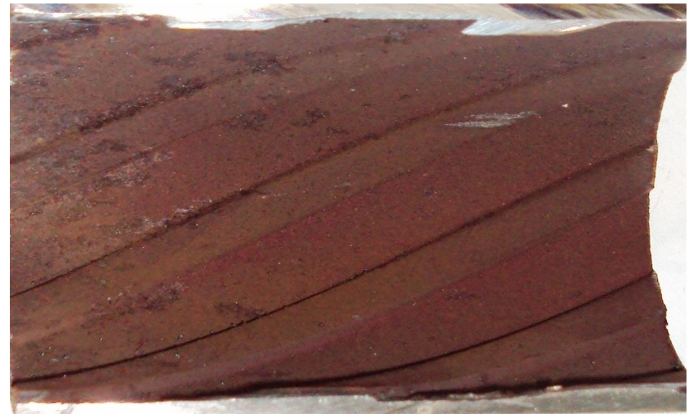
\text{FeOOH}/\text{Fe}_2\text{O}_3 block pores lowering \text{Fe}^{2+} migration
