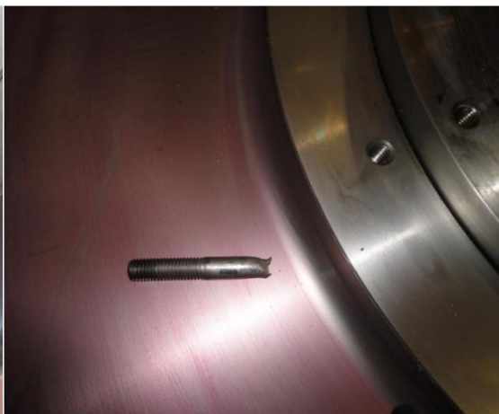
Broken bolt found the section of discharge cover
