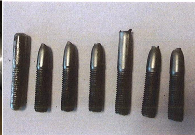
Broken bolts after remove
