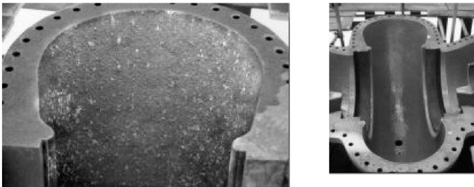
Figure 7.10 – Surface of a Pump Casing before and after a Finished Coat
