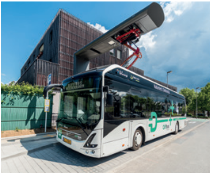
The Netherlands is home to a number of international suppliers of smart charging infrastructure and services, including Alfen, EVBox, Allego and Greenflux. Heliox focuses on charging solutions for public transport, and recently unveiled the world's first battery-integrated charging station for fast-charging e-buses and e-trucks.
