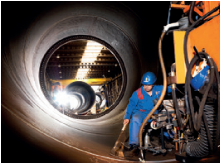
Sif Group is a global leader in monopile foundations for offshore wind farms. It is already manufacturing the huge monopile foundations required for larger turbines, with a diameter of up to 11 metres and a maximum weight of 2,000 tonnes.
