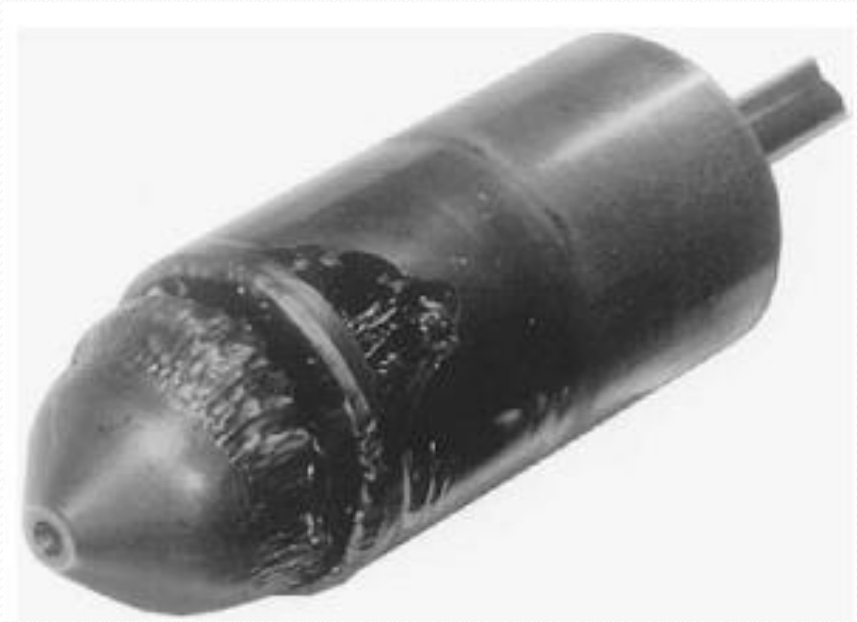
Plug damaged by flashing
