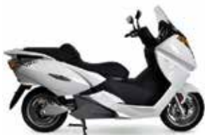
Fig. 14. Battery scooter (Vectrix Corp, 2010) Battery: Li: LiFePO 4 , 30Ah capacity
