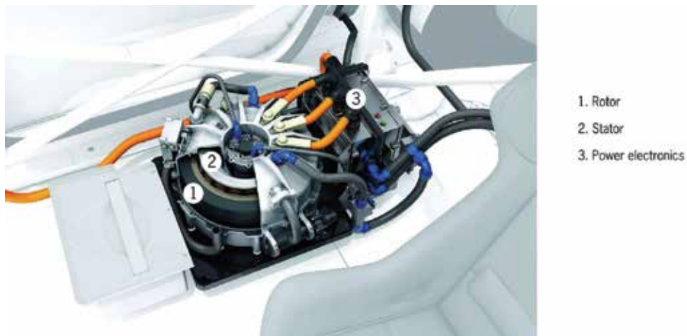
Fig. 3. FES system in a high-performance hybrid automobile (courtesy of Dr. Ing. h.c. F. Porsche AG, Stuttgart, Germany)
