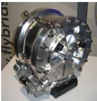
Fig. 32. The Jaguar flywheel module with integrated vacuum and lubrication pumps (Flybrid Systems, 2010)
