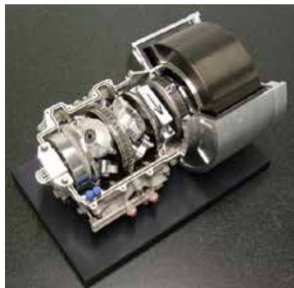
Fig. 31. The original CVT based Formula One KERS (Flybrid Systems, 2010)
