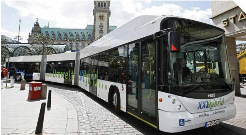
Fig. 19. The hybrid bus with supercapacitors (Maxwell Technologies, 2011)
