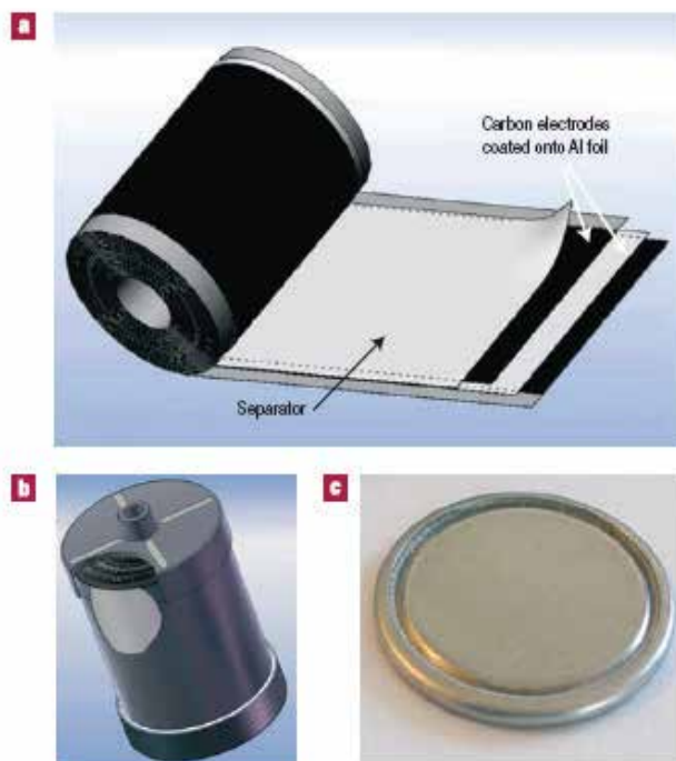
Fig. 9. a) Schematic representation of a double-layer spiral capacitor; b) assembled device (500 grams, 2600 F); Batscap, Groupe Bolloré; c) button cell (1.6 mm height, 5 F capacity); Y-Carbon.
