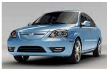
Fig. 15. Battery car (CODA Automotive, 2010) Battery: LiFePO 4 , 728 cells (104s7p)
