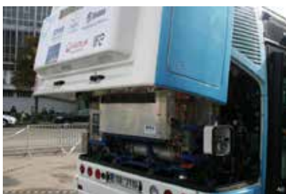
Fig. 2. Detail on fuel cells, the ESS is composed of Li-ion battery and supecapacitors (TriHyBus.cz, 2008)
