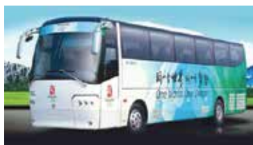
Fig. 16. Battery bus (Zhongtong Bus Holding Co, (n.d.) Battery: Li-ion, 540 Ah capacity
