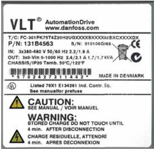
Fig 9.2 Identification data of a Danfoss frequency converter
