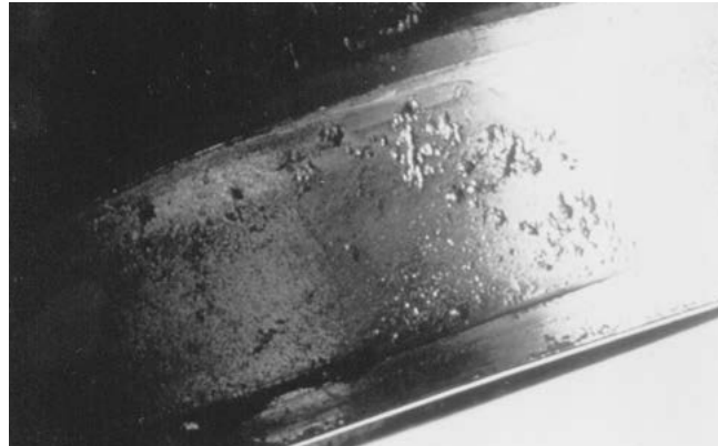
Figure 7. Spalls & Wear Patterns in the Race
