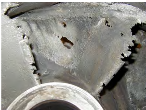
Figure 1. Cavitation damage to an impeller.
