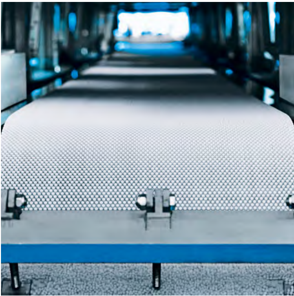
Figure 6. IPCO's paraffin wax pastillation process.
