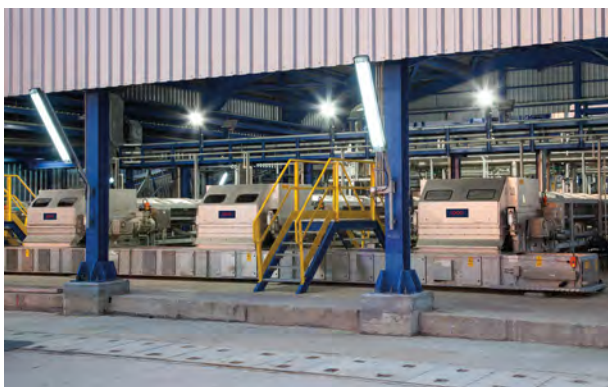
Figure 1. Discharge end of Rotoform HS pastillation units.
