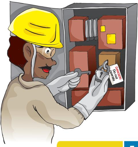
Lock out and tag out hazardous equipment in a confined space.
