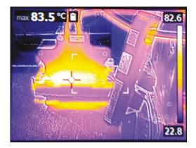
**Figure 11.** Temperature measurement of the second developed MFT with split windings at power of 45 kW without forced cooling.
