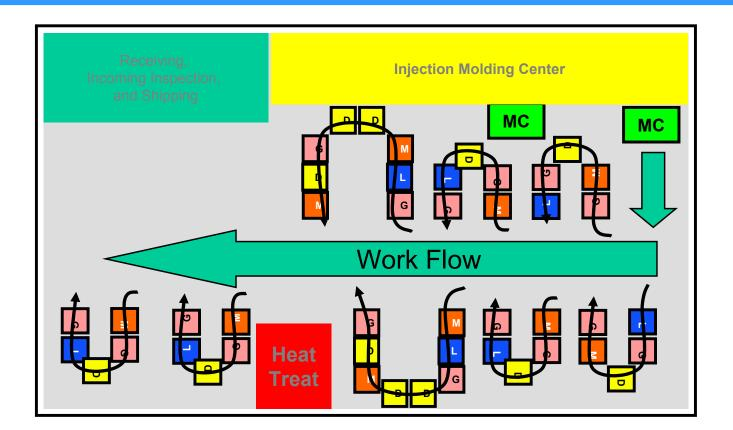
Rather than route the materials required through the entire plant, materials flow to the head of each work cell, through each process in the cell, then to final assembly. This eliminates most of the transportation and waiting we would see in the traditional approach.
