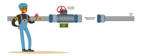
The disadvange with this method is that, if the pipe is large, it is difficult to remove the spool. In addition, lifting equipment and more manpower are needed to achive isolation.
