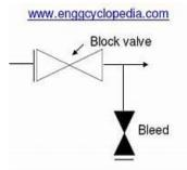
DBB can be two seprated block valves and and one bleed valve OR a single unit in a compact design.
