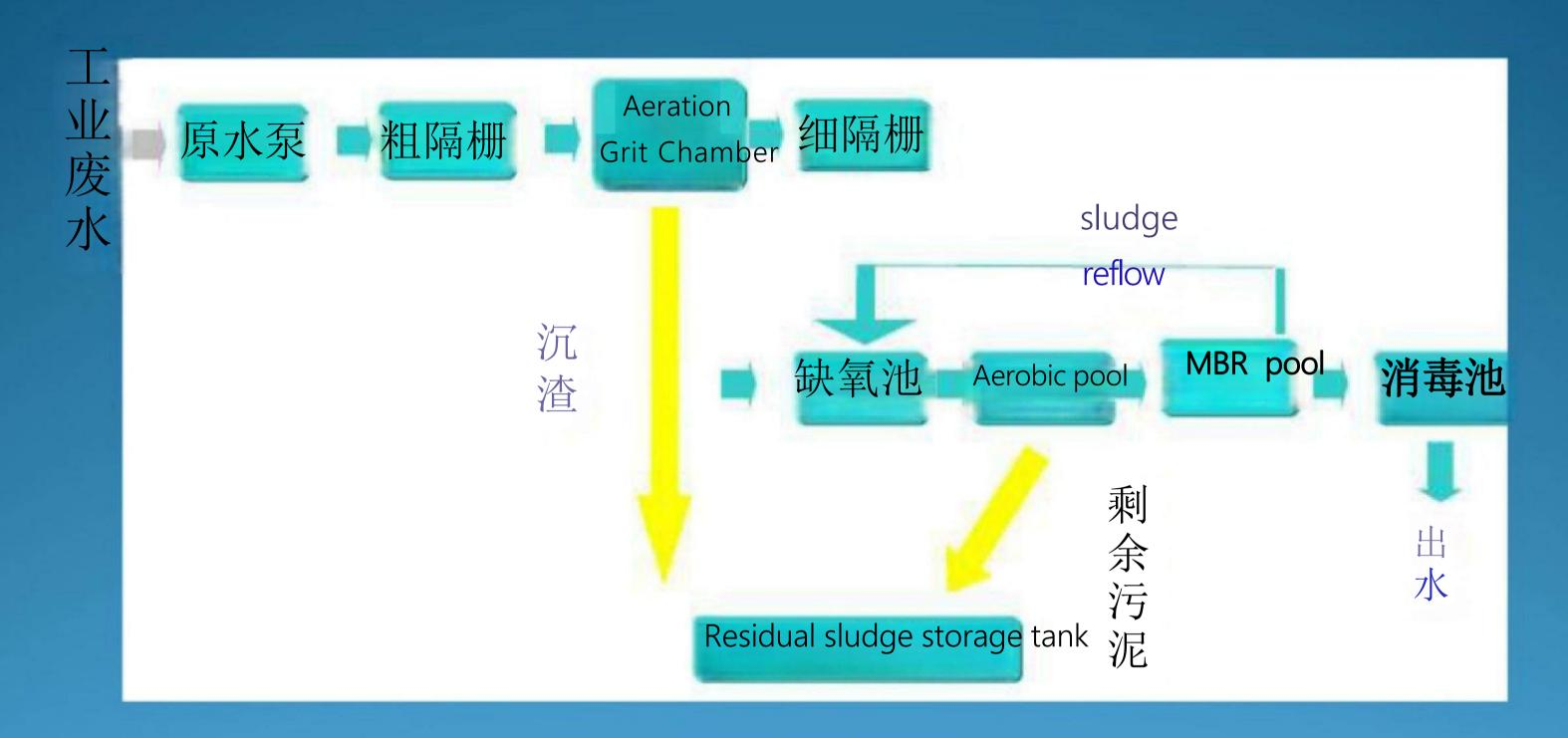
The recommended process for the removal of organic matter in industrial wastewater
