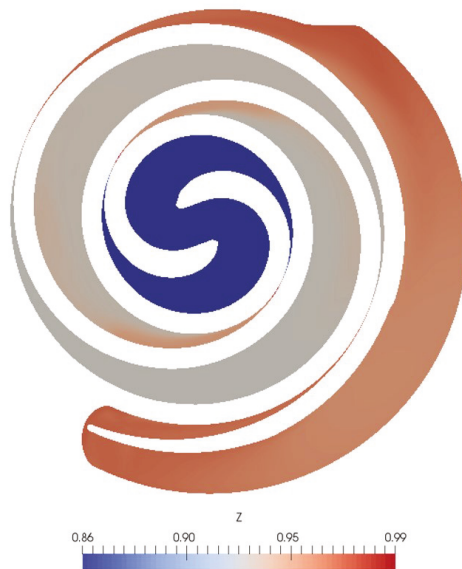
Figure 6. Compressibility factor for R134a during the operation of the expander.
