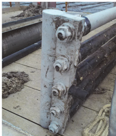
Figure 9.48 Example of aerated lagoons in operation at a large facility. Above is a view of the lagoon from the effluent side; on the left shore is the air manifold with all the floating headers where many diffuser assemblies are attached and floating underwater. Bottom left is an image of the blower house. Bottom centre is a photograph of a damaged assembly being retrieved on the service barge; note the large amount of rags being removed from the surface of the assembly, visible on the left and at the top of the image; one of the diffuser membranes was removed from this assembly for off-site fouling studies. Bottom right is a detail of the said diffuser membrane surface.
