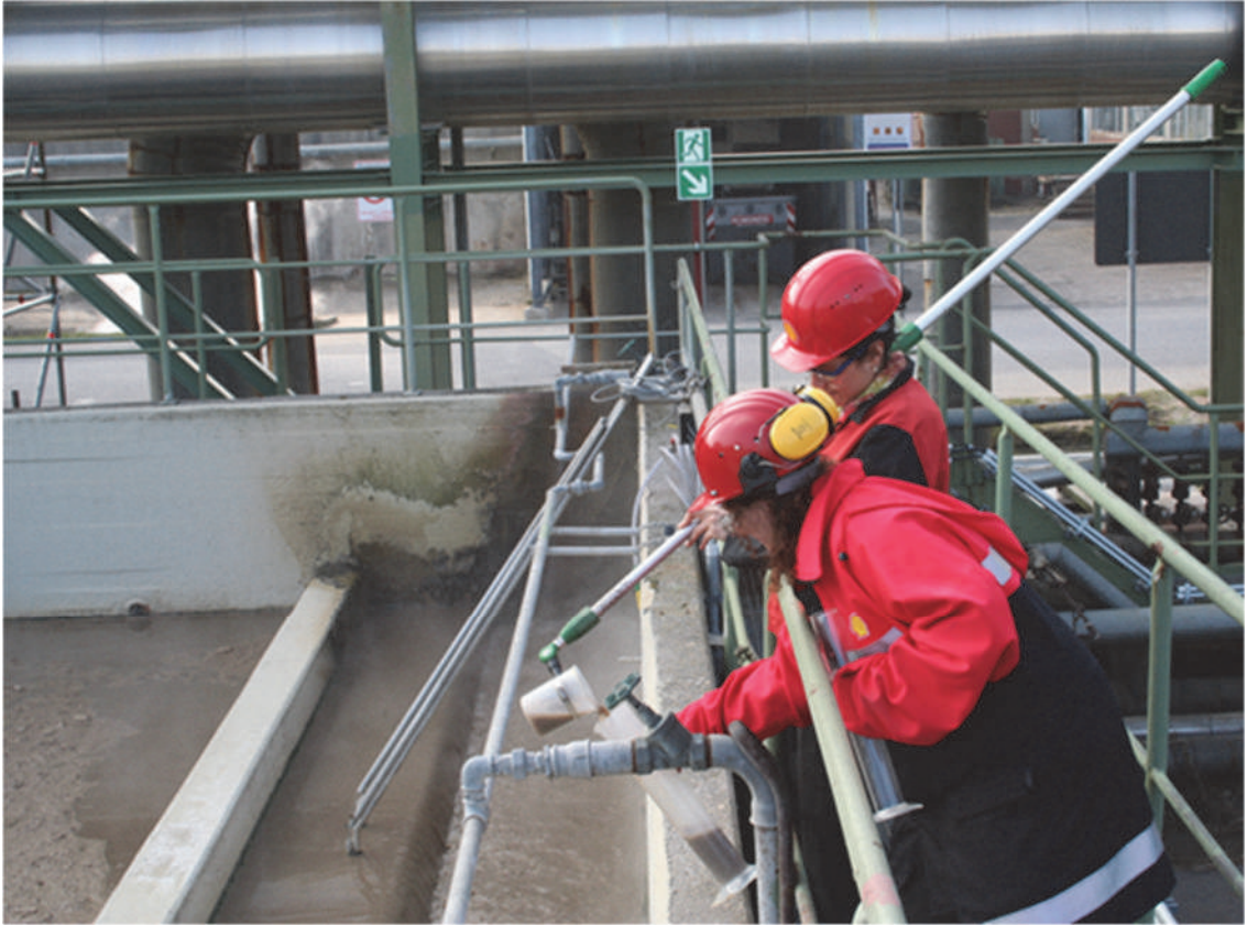
Figure 3.19 Sampling is an essential part of wastewater and sludge characterization. The photo shows sample collection from an oil refinery wastewater treatment plant (Photo: D. Brdjanovic).
