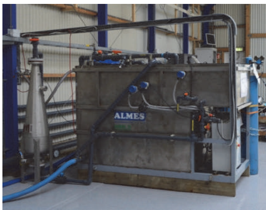
Figure 13.32 The pilot-scale Speece cone HL-MBR system located at the Harnaschpolder wastewater treatment plant in Den Hoorn, The Netherlands. On the left-hand side of the photo is the Speece cone aeration device, and on the right-hand side is the MBR (photo: H.A. Garcia).
