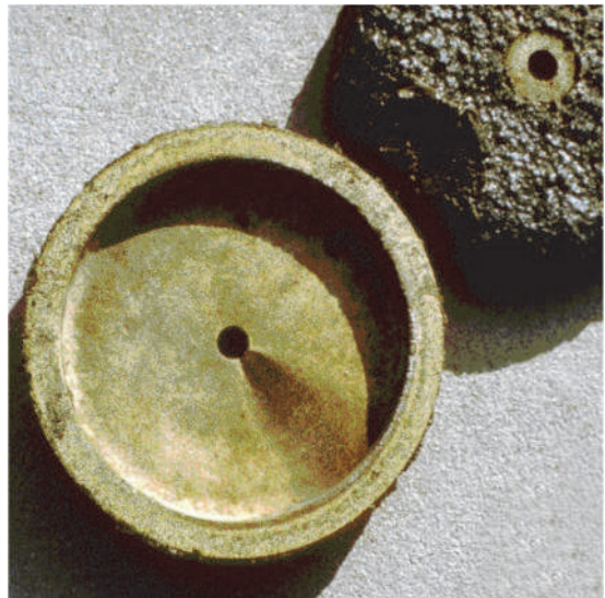
Figure 9.4 The first generation of fine-pore diffusers: ceramic domes (top). Air is fed through a hollow bolt, filling the space enclosed by the dome, and is then released through the pores of the sintered ceramic. On the bottom is a diffuser harvested after a prolonged time in operation, with visible bio-fouling on the outer surface. The discoloured section of the dome interior shows the position of the bolt's air release hole and is due to contaminants in the air supply.
