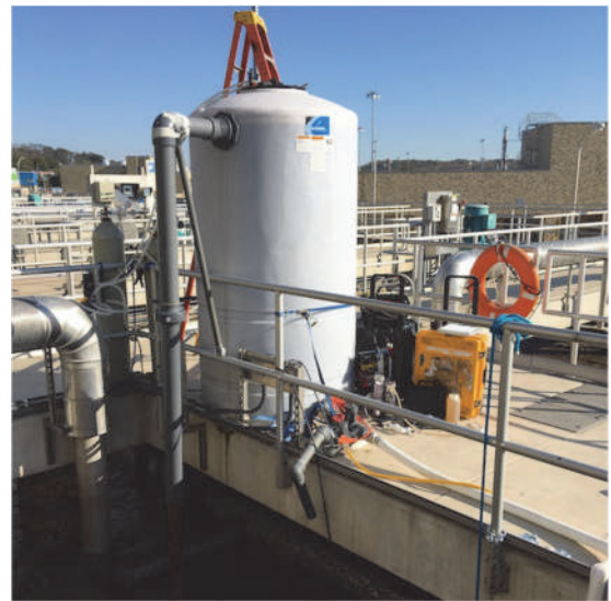
Figure 9.39 Schematic and image of in-situ column testing for process water.
