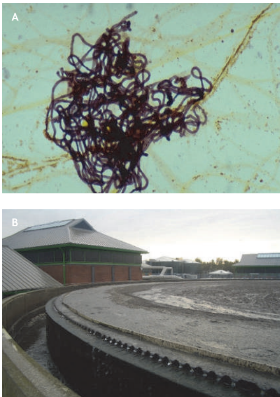
Figure 10.3 Nightmares for the wastewater treatment plant operator: (A) filamentous bacteria, (B) bulking sludge leaving the plant with the effluent (photos: D.H. Eikelboom and D. Brdjanovic).
