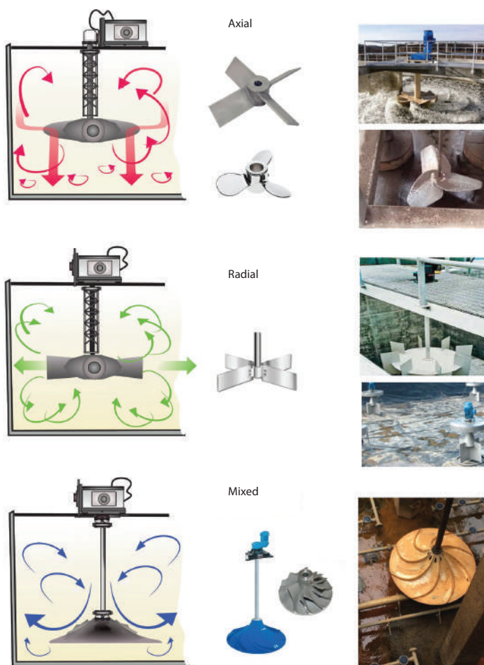
Figure 9.23 Schematics of flow patterns and image of different impellers.
