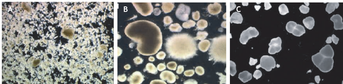
Figure 18.9 Development of aerobic granular sludge in a sequencing batch airlift reactor started up with conventional activated sludge after (A) 4, (B) 13, and (C) 87 days of reactor operation (photos: M.C.M. van Loosdrecht).
