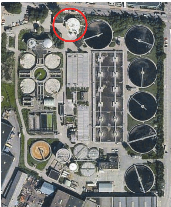
Figure 5.25 WWTP Beverwijk; the red circle shows the area used for the SHARON® process that treats 1,200 kg nitrogen per day.
