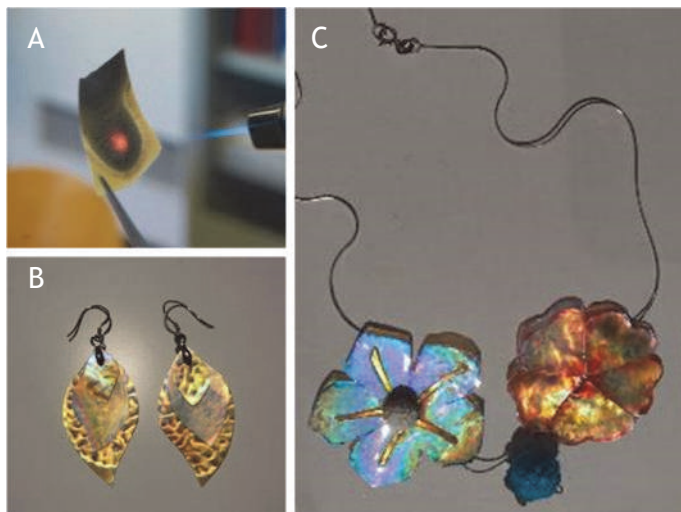
Figure 11.18 A: Flame-retardant composite plastic derived from Kaumera and clay. B and C: wastewater-based earrings and necklace. The main material is Kaumera and cellulose composite. The plastic sphere on the necklace is from PHA. The blue colour is vivianite and the red colour is extracted from anammox sludge (art created by Yuemei Lin).
