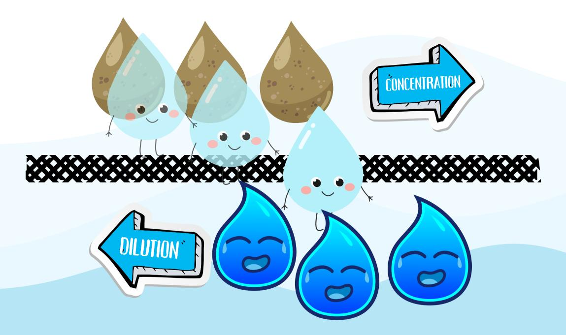
NOW, THE WATER IN THE DIRTY SOUP LIKES THE SALT WAY MORE THAN THE DIRT. IT FLOWS OVER ON THE OTHER SIDE OF THE FILTER. SINCE THE SALT WATER ATTRACTS THE WATER IN THE DIRTY SOUP, WE CALL THE SALT WATER THE "DRAW SOLUTION".
