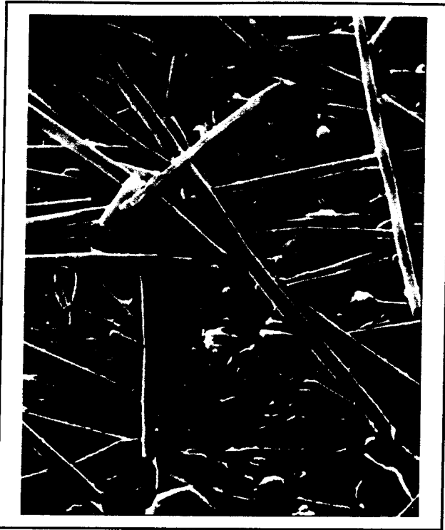
Figure 2.8 Suspended Solids Filtered from Aegean Seawater Magnification = 1000 x (Courtesy Brown & Root, Inc.)
