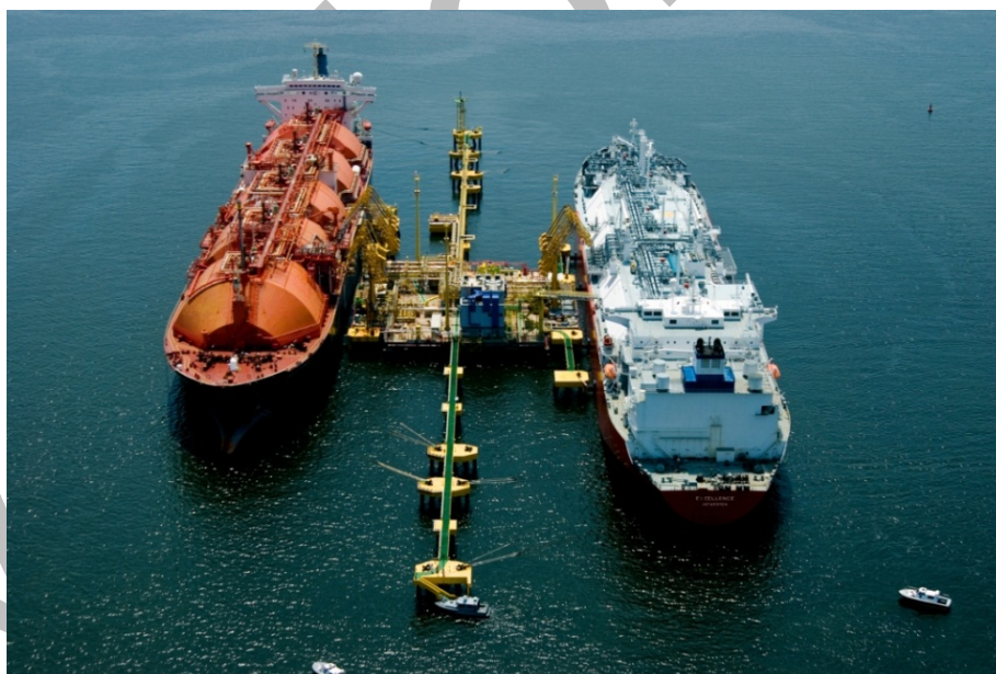
Figure 4-2 Cross-dock transfer arrangement [Source: Petrobras]
