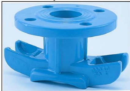
Fig 7.6: Universal drill-clamp with flange pipe size 2" DN 40/50 PN 4 / 58.0 psig (gas) / PN 16 / 232.1 psig (water)
