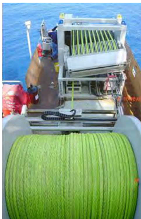
Figure 4. Logan's work on Perdido was the first time that Shell had ever used this type of soft rope winch system for its oil and gas production.
