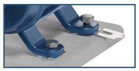
This completes the final soft foot check. This will ensure that there is no unintended movement during the more precise steps of shaft alignment.
