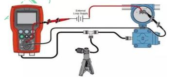
We have to use HART communicator. Connect the communicator with the transmitter select the HART Communicator Menu for lower
