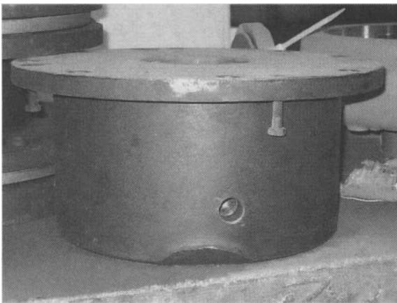
Figure 14.2: Coupling hub damaged with severe hammer blows at disassembly.
