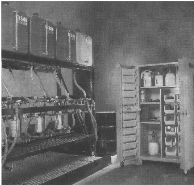
Figure 12.7: Minibulk storage indoors. Note approved transfer containers on upper shelf of cabinet (Ref. 3).
