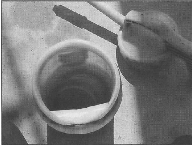
Figure 12.3: Careless handling of an approved transfer container can still cause extreme particulate contamination (Ref. 3).
