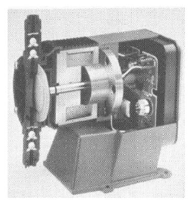
Larger diaphragm pumps may be operated by mechanical means in a fashion similar to the piston pump. The biggest difference is the replacement of the piston with a flexible diaphragm. The diaphragm is attached to a metal rod that is operated by an eccentric cam driven by an electric motor.
