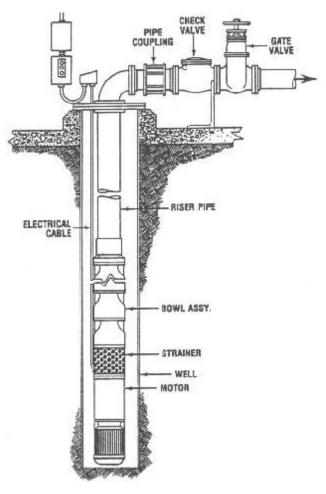
requirements. Standard construction includes cast iron bowls with bronze impellers on a stainless steel pump shaft. A suction strainer is used to prevent foreign objects from entering the pump.
