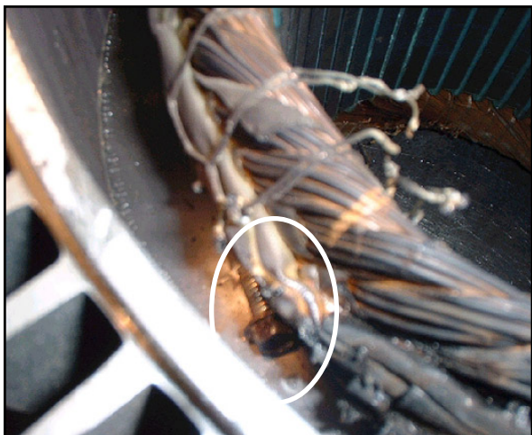
Loose laminations, low slot fill, phase insulation out of place and improper full-slot lap winding method.
