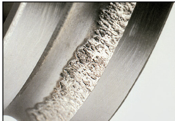
Severe spalling caused by excessive load. This spalling is part of the natural failure process as a bearing reaches the end of its life.
