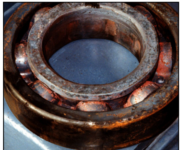
The lubricant was washed out of the bearing. Rust is evident.
