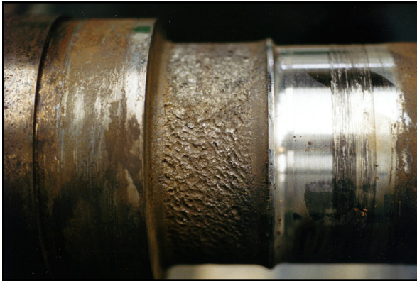
These shafts show signs of a classic case of excess radial load on a ball bearing.
