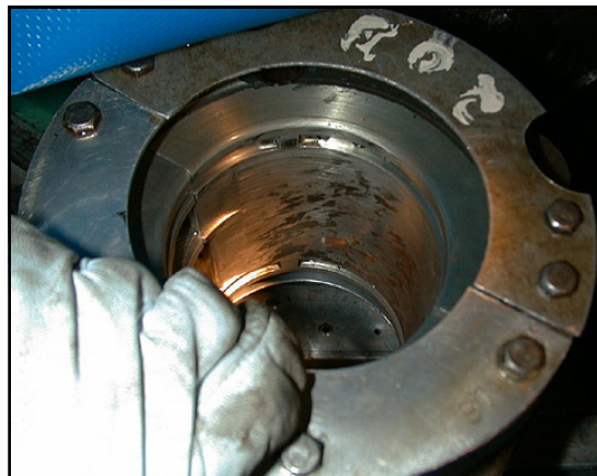
FIGURE 32: OIL DISTRIBUTION GROOVE TOO SMALL
