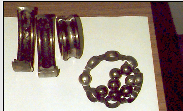
Above, the side of the bearing toward the rotor has been marked prior to dissection. Below, a dissected ball bearing.
