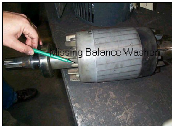
The balancing weight was not properly secured to the rotor nib and eventually was thrown into the stator winding causing a turn-to-turn short.
