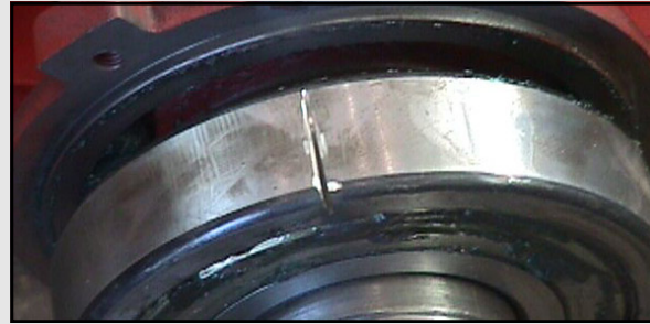
Above, the side of the bearing toward the rotor has been marked prior to dissection. Below, a dissected ball bearing.
