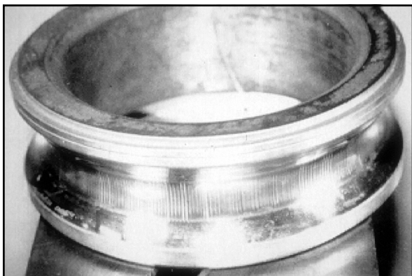
Fluting due to shaft currents on both a roller bearing, above, and a ball bearing, below.
