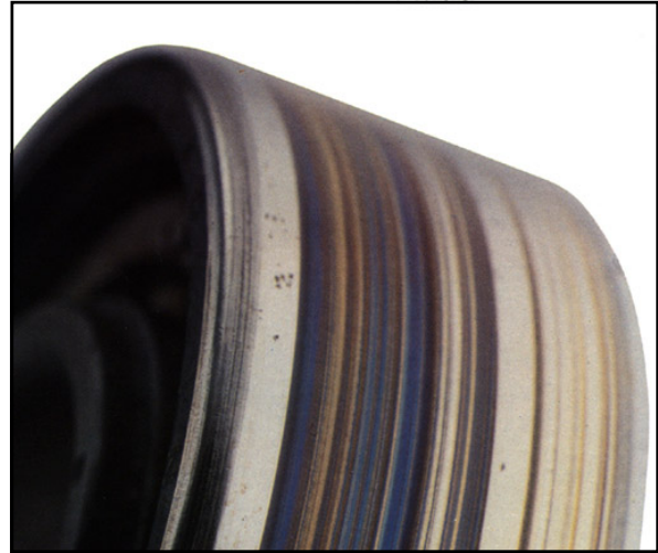
Discoloration and scoring is the result of the outer race slipping in the bearing housing.
