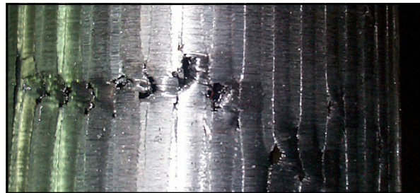
Voids located near the surface of the rotor. This rotor was machined to expose the voids.
