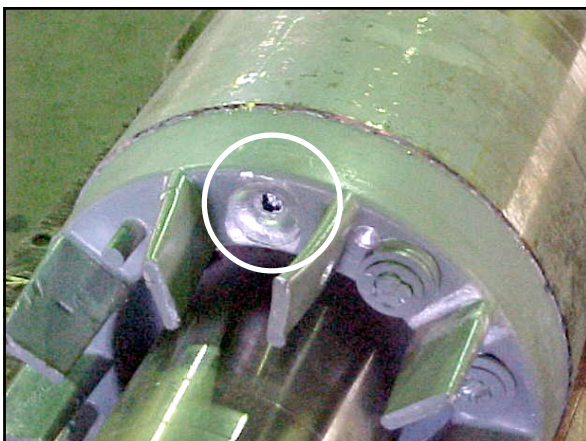
Balancing nib broke loose at the point highlighted above.
