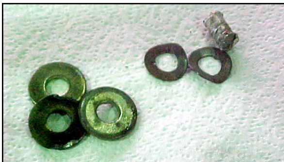
Broken balancing nib and balancing weights.
