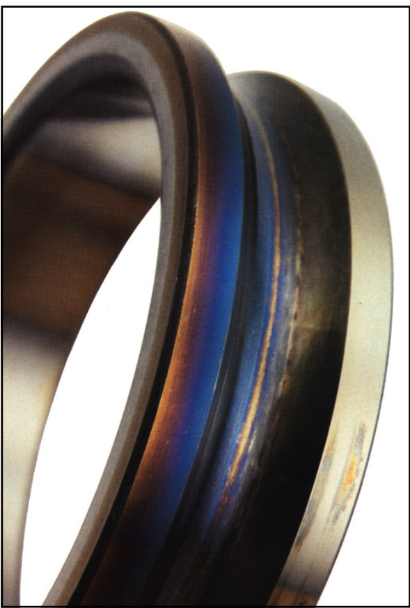
Symptoms of overheating are discoloration of the races, balls and cages from straw to blue. Temperatures in excess of 400° F (205° C) can anneal the race and ball materials. The resulting loss in hardness reduces the bearing capacity, causing early failure. Courtesy of The Barden Corporation
