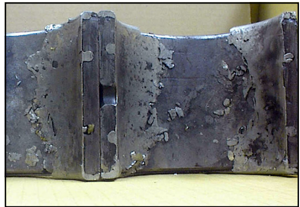
Examples (above and below) of babbit fractured by high vibration and/or impact damage.
