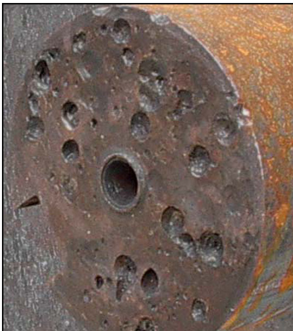
Contamination from moisture or chemicals trapped in the coupling arrangement eroded the surface of the shaft.
