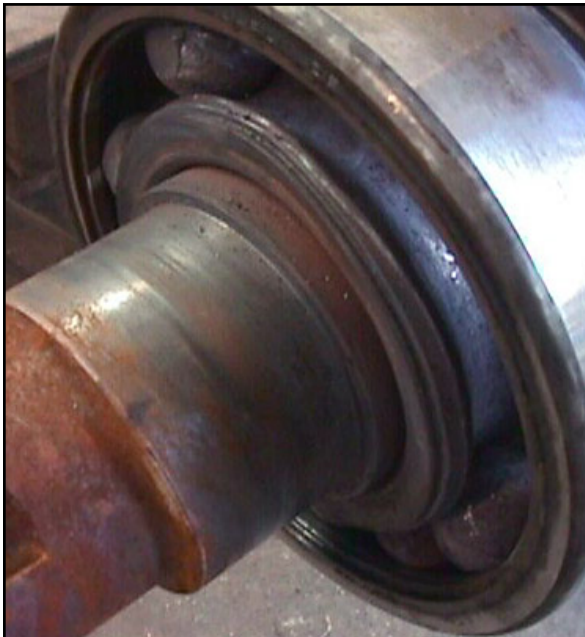
Grease was flushed from this bearing. Water, steam or solvents are often the cause of this type of damage.
