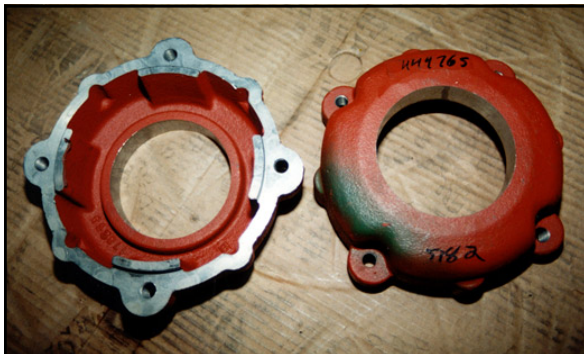
Note the contrast between a proper fitting bearing cap that is in good condition (left) and those that are no longer functional (right).
