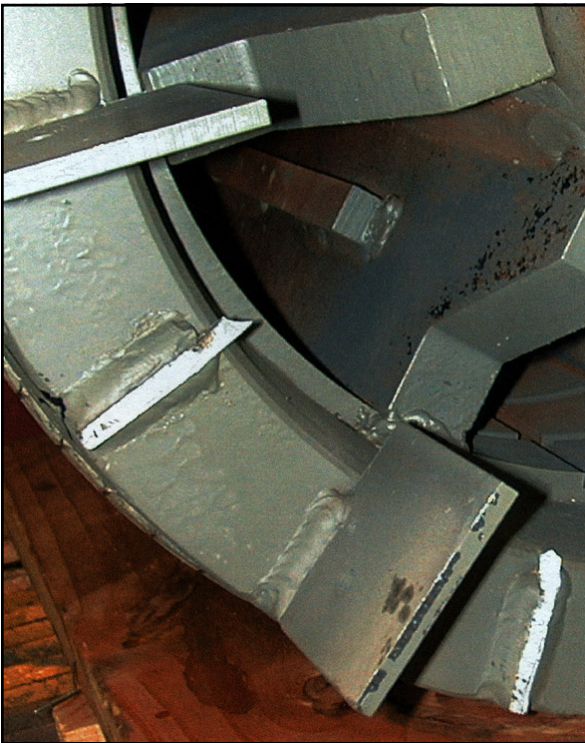
The rotor fan blades fractured above the welds due to cracks and vibration that resulted from fatigue in the aluminum.
