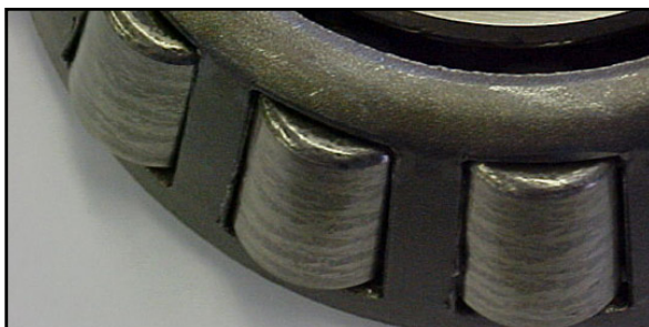
The irregular striped discoloration was caused when contamination was pressed in the roller path.
