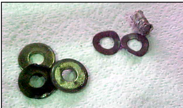
Broken balancing nib and balancing weights.
