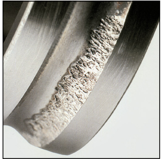
FIGURE 14: SPALLING ON A BEARING RACEWAY
