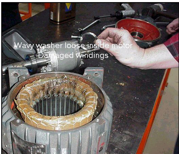
A bolt (top) or washer (middle) dropped during motor assembly, or a washer that comes loose during operation (bottom), can cause a ground failure. Be sure to account for all the bolts, nuts and other hardware.
