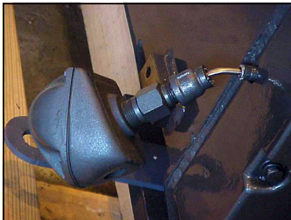
This bearing resistance temperature detector (RTD) was damaged during shipping.
