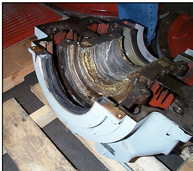
The failed drive end sleeve bearing.
