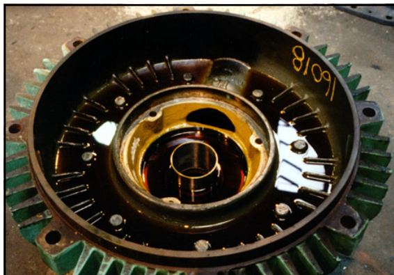
FIGURE 23: OIL POOLED IN THE BOTTOM BRACKET
