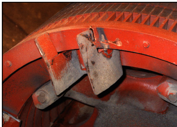
The bolts that held these fan blades in place on the end ring “worked” loose.
