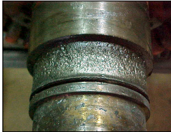
These shafts show signs of a classic case of excess radial load on a ball bearing.
