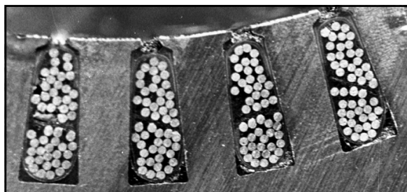
This stator shows signs of loose coils and low slot fill. Loose wires will vibrate in the slots causing chafed insulation and fatigue fractures. Note the poorly positioned separators, the extra space at the bottom square corners and the voids. Heat transfer also suffers. Filler spacers, more copper or better varnish retention would improve this winding.
