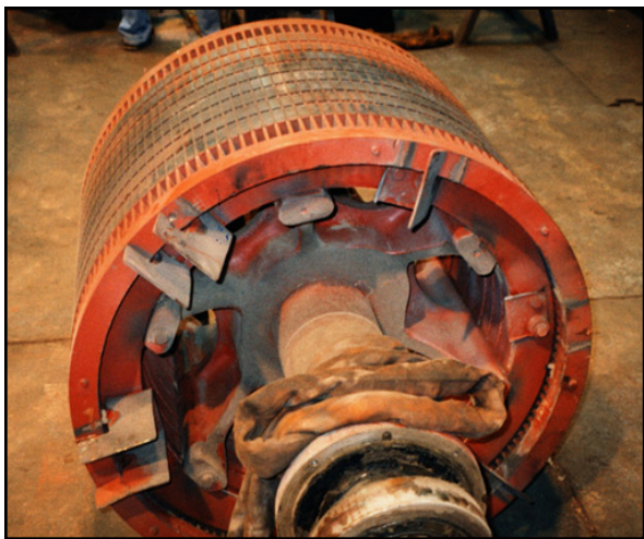
The bolts that held these fan blades in place on the end ring “worked” loose.
