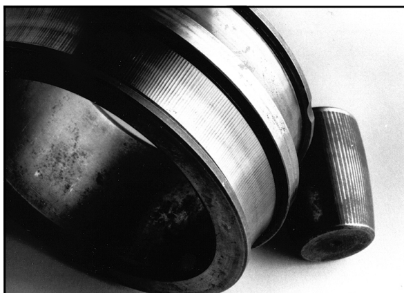
Fluting only occurred on the non-loaded roller path because the arcing occurred only at the gap between the rollers and the race. A good analogy is the points in an older automobile ignition system.
