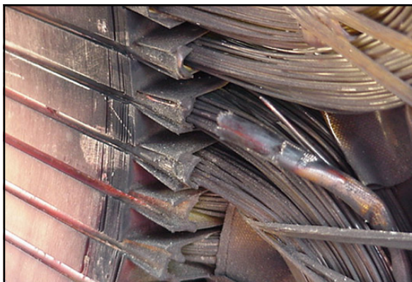
Loose laminations, low slot fill, phase insulation out of place and improper full-slot lap winding method.
