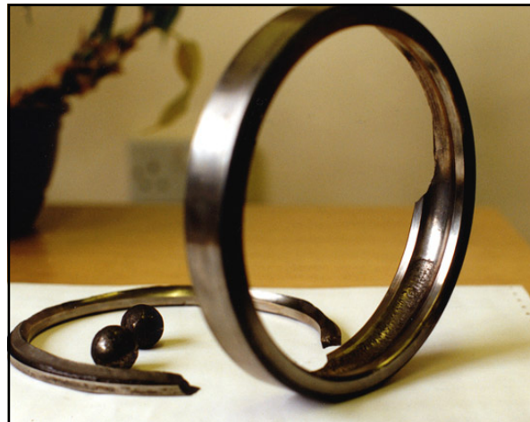
Heavy shock loads can cause unusual fractures of the outer race and/or balls.
