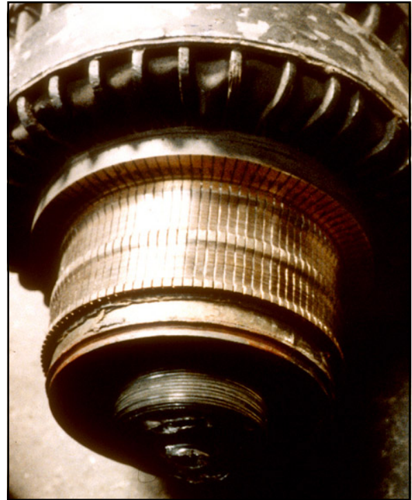
Grooving is caused by abrasive wear by either dust in the atmosphere or too abrasive a brush grade. The two major problems associated with grooving are:
