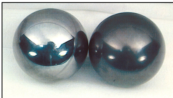
When rotational speed varies, the shaft currents may cause a dull, frosted appearance instead of fluting.
