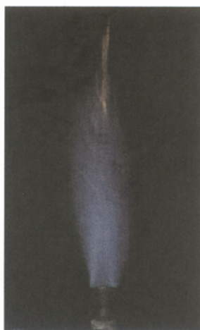
Figure 35b Good pilot flame.
