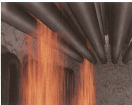
Figure 14 Flames should never strike furnace tubes, as they are shown doing in this figure.
