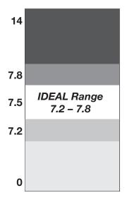
Pool water pH is best kept in the range of 7.2 to 7.8. When pH remains below 7.2, the water is considered to be corrosive. This means etching of plaster and metals in equipment such as heat exchangers will result. In addition, it is more difficult to keep chlorine in the pool because while more effective as a sanitizer at the low pH, chlorine is also much less stable resulting in the consumption of larger quantities of chlorine than would be used at normal pH levels.
