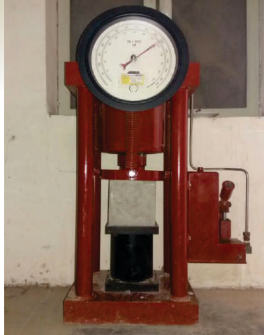
Figure-3.16 Compression Testing of Sample Cube
