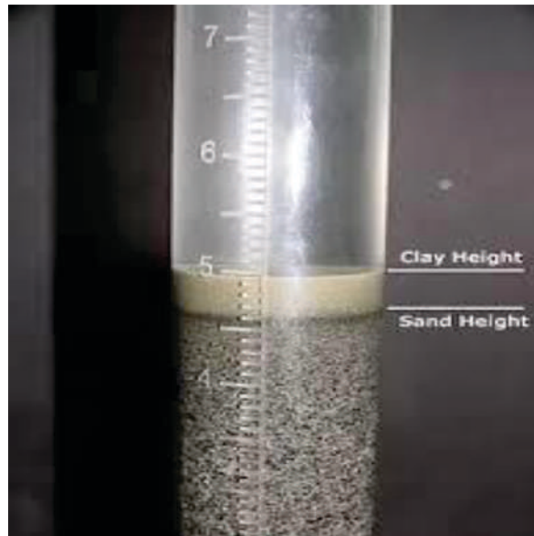
Figure-3.4 Testing sand for silt contents
