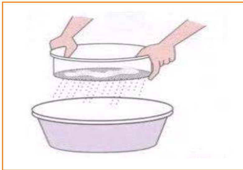
Figure-3.3 Manual Sieving of Aggregates
