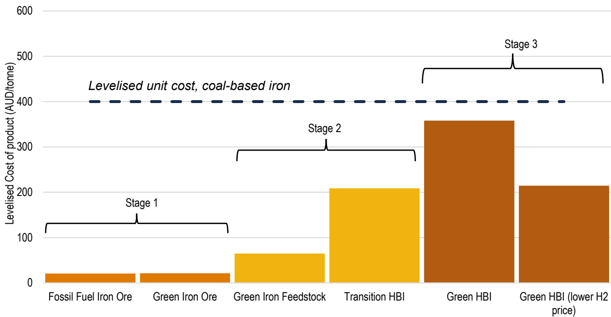
Figure ES17 Levelised cost of production for Green Iron in the form of HBI transition strategies using hematite ores
