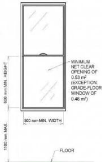
FIGURE 1030.2 EMERGENCY ESCAPE WINDOW
