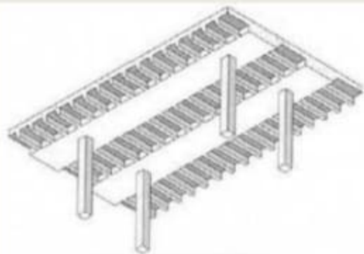
Figure 5A-2. Joist floor system on wide shallow beams
