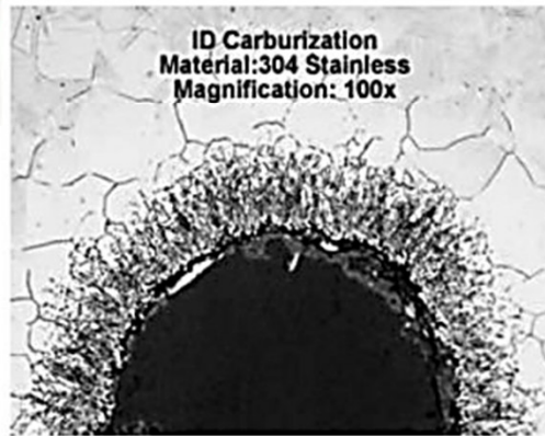
1- Close-up of pit shown in Photograph 10. The black material in the bottom of the pit is coke. The smaller pits (at arrows) are smaller versions of the large pit.
