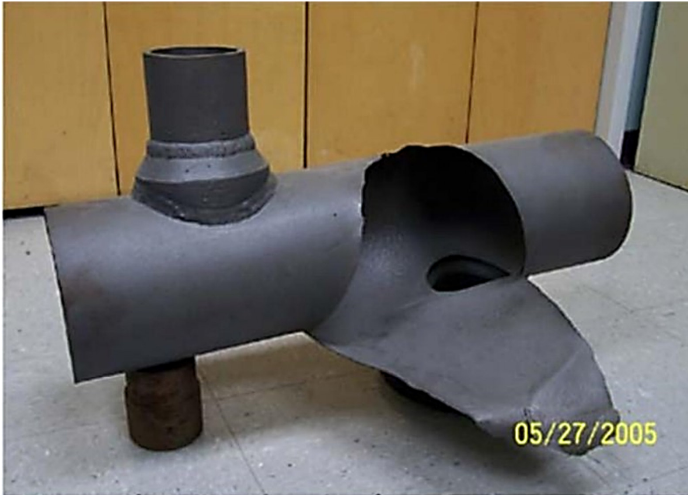
Figure 4-116 – Sulfidation failure of NPS 8 carbon steel pipe. Note the relatively uniform thinning that resulted in a sizeable rupture.
