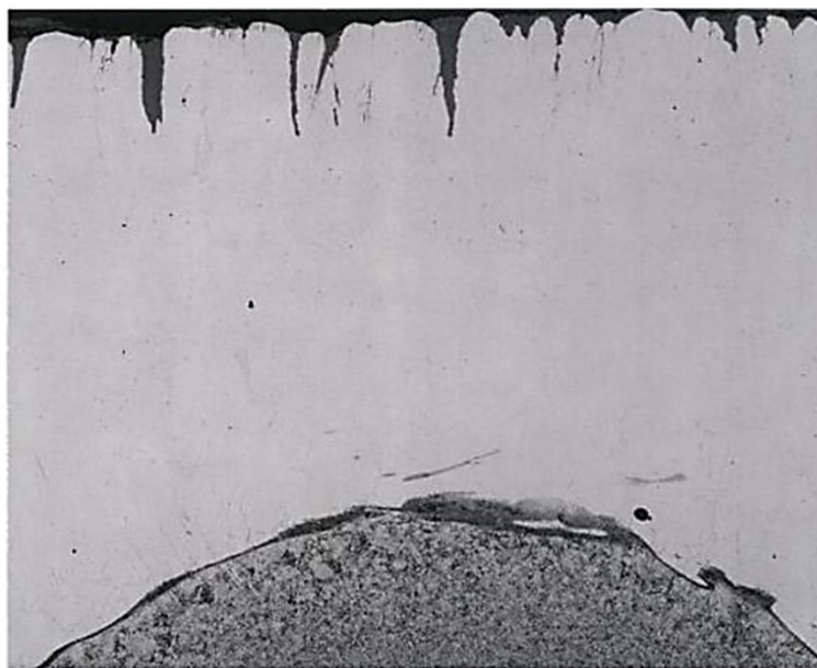
Figure 4-129 – On waterwall tubes, even with a corrosion-resistant weld-overly, circumferential cracking will develop. Mag. 37½X, etched.
