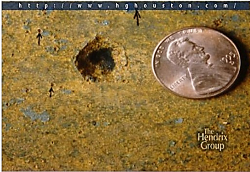
1- Close-up of pit shown in Photograph 10. The black material in the bottom of the pit is coke. The smaller pits (at arrows) are smaller versions of the large pit.
