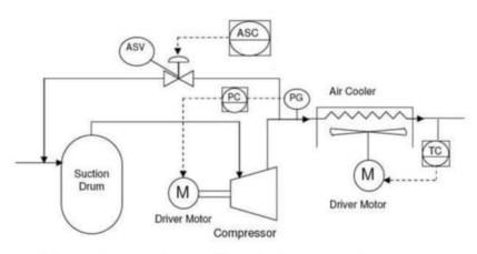
ASC : Anti Surge Controller ASV : Anti Surge Valve TC : Temperature Controller PC : Pressure Controller
