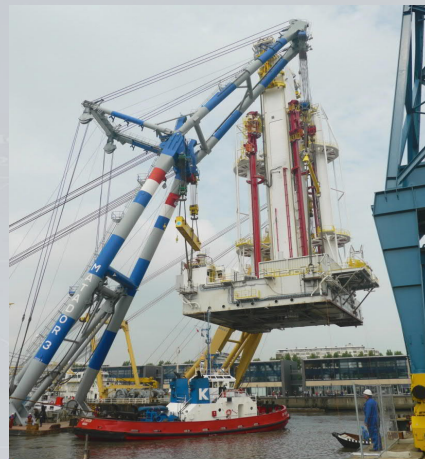
Lifting a 2400 Tons Drill Tower with 2 Floating Cranes
