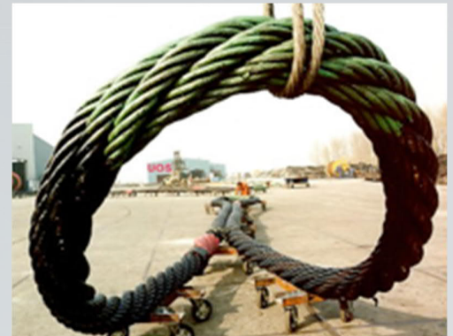
Offshore Grommet made of 300 mm diam. wire rope
