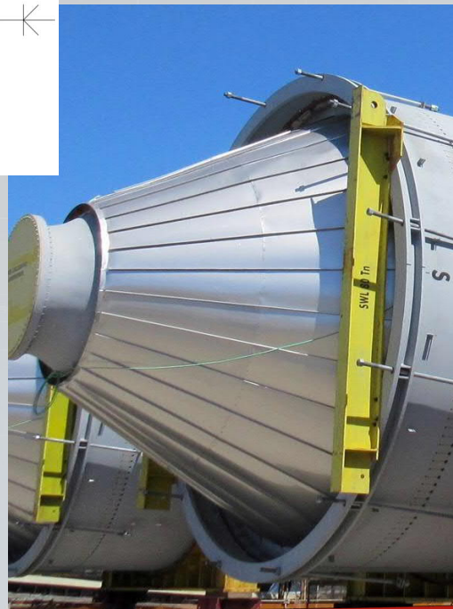
Tailing frame bolted to the skirt
