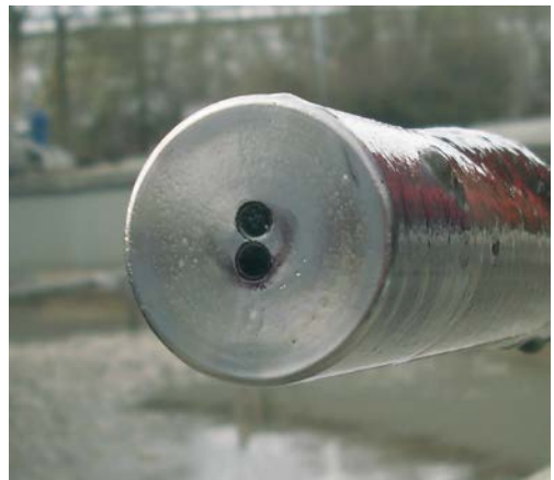
ViSolid® 700 IQ with working ultrasonic cleaning system shows no adverse effect.
