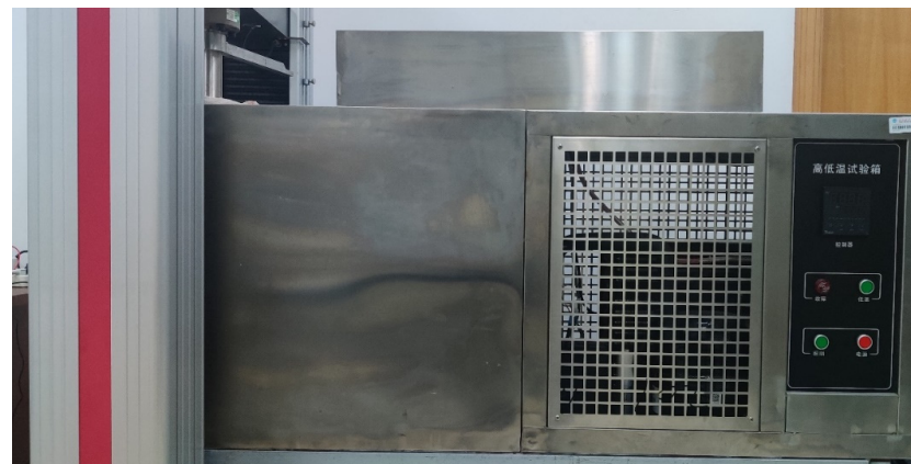
Figure 5. Low-temperature test chamber.
